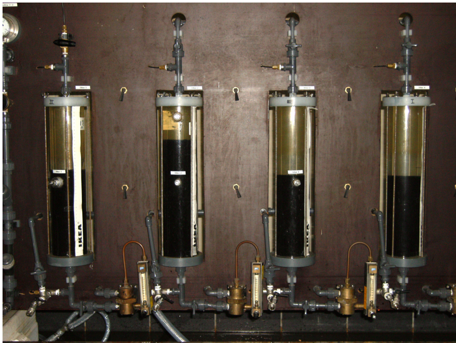
Figure 28: Expansion of the filter bed when backwashing filter 2.
