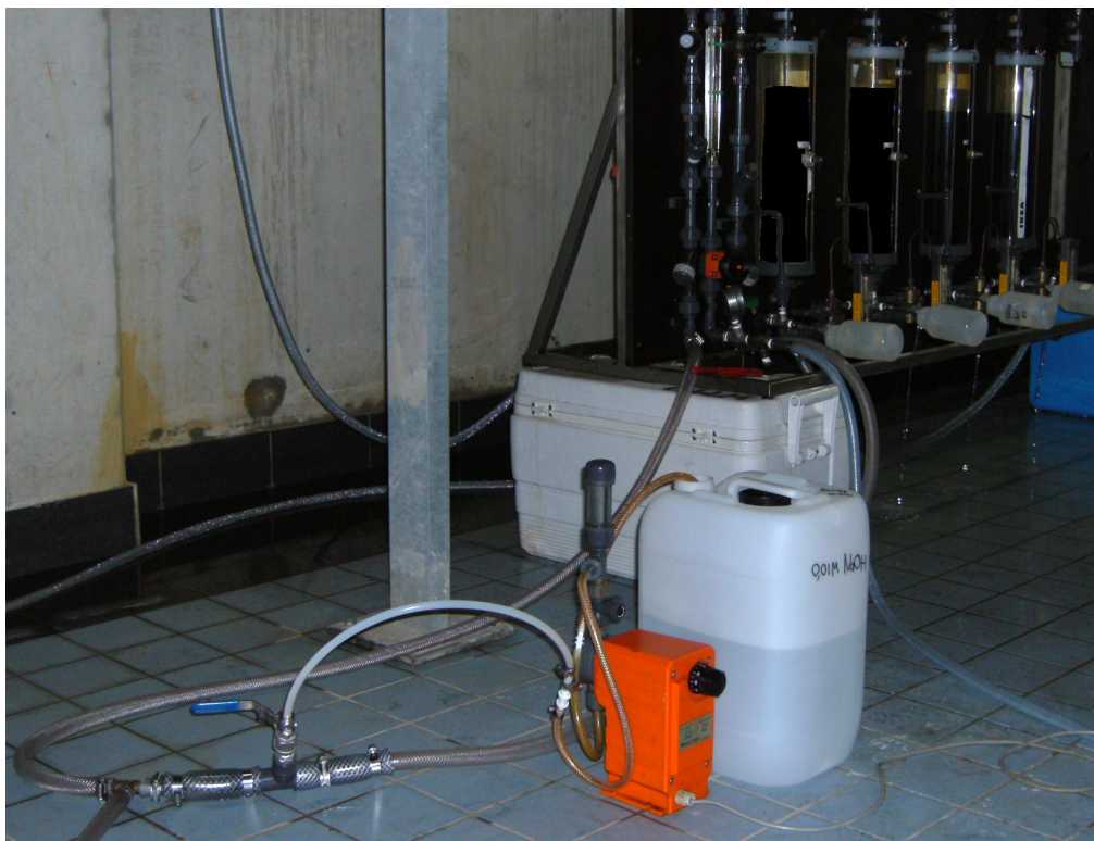
Figure 26: Experiment with caustic soda dosage to column 1 and 2.
