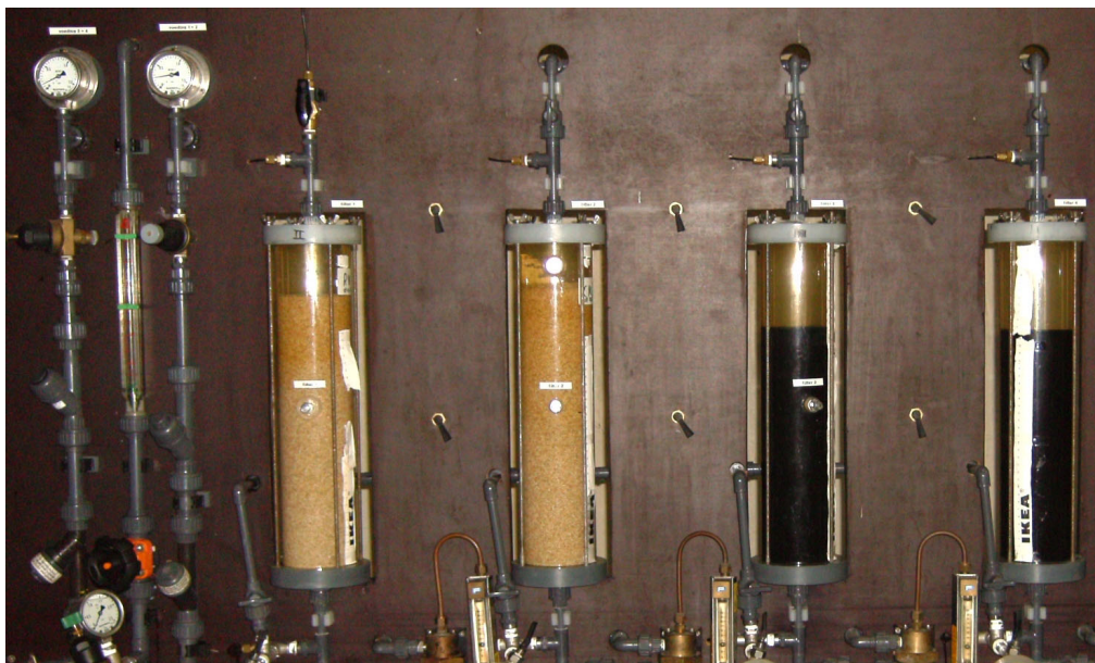
Figure 27: Experiment with crushed limestone filtration in column 1 and 2.
