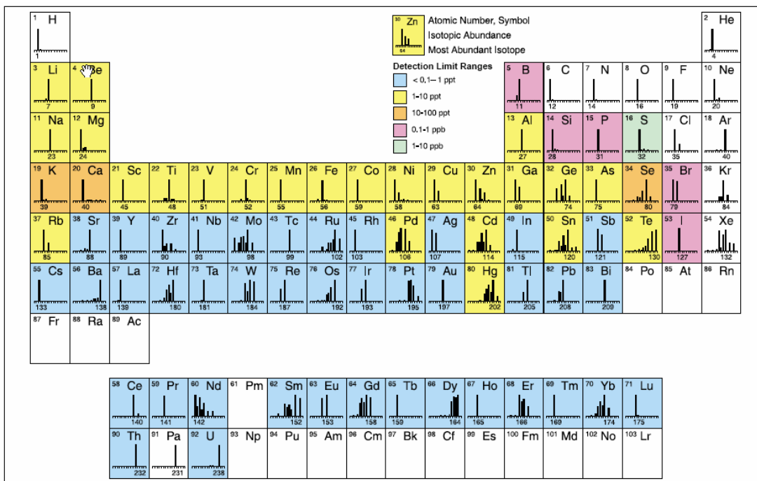
Figure: Approximate detection capabilities of the ELAN 6000/6100 quadrupole ICP-MS (Courtesy of PerkinElmer, Inc.)
