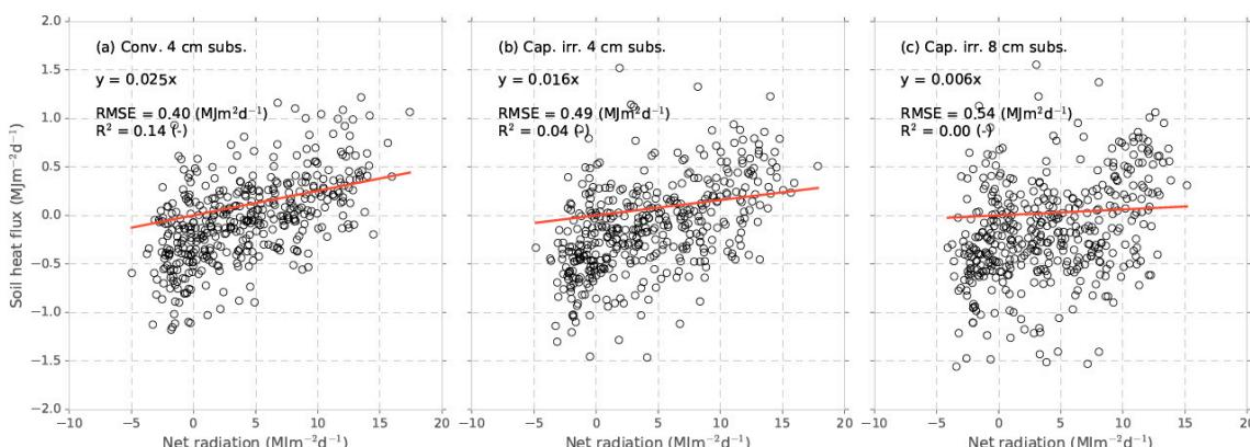
**Figure A1.** Linear regression between on-site measured net radiation  $R_n$  and soil heat flux  $G$ .
