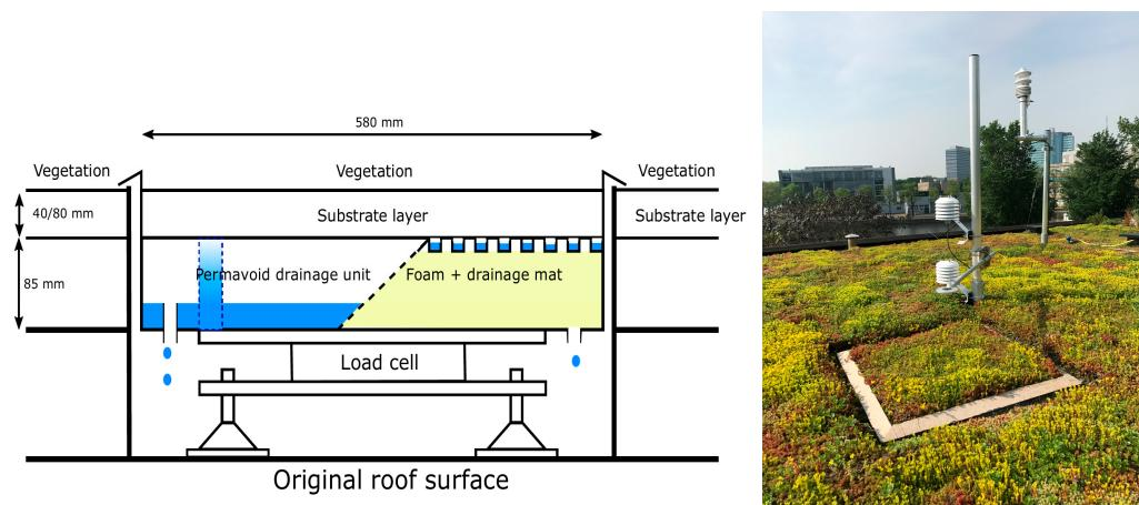
**Figure 3.** Lysimeter design (left), and (right) a lysimeter embedded in the green roof surface shortly after planting the sedum blankets. The drawing of the lysimeter shows the two roof designs: storage and capillary irrigation (left of the diagonal dashed line) and a conventional build up (right of the diagonal dashed line).
