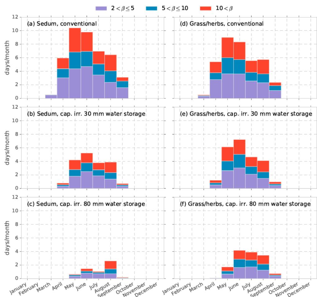
**Figure 10.** Long-term energy performance of green roof systems expressed in an average number of days per month within a certain Bowen ratio range. The total height of the stacked column denotes the average number of days per month with  $\beta > 2$ .
