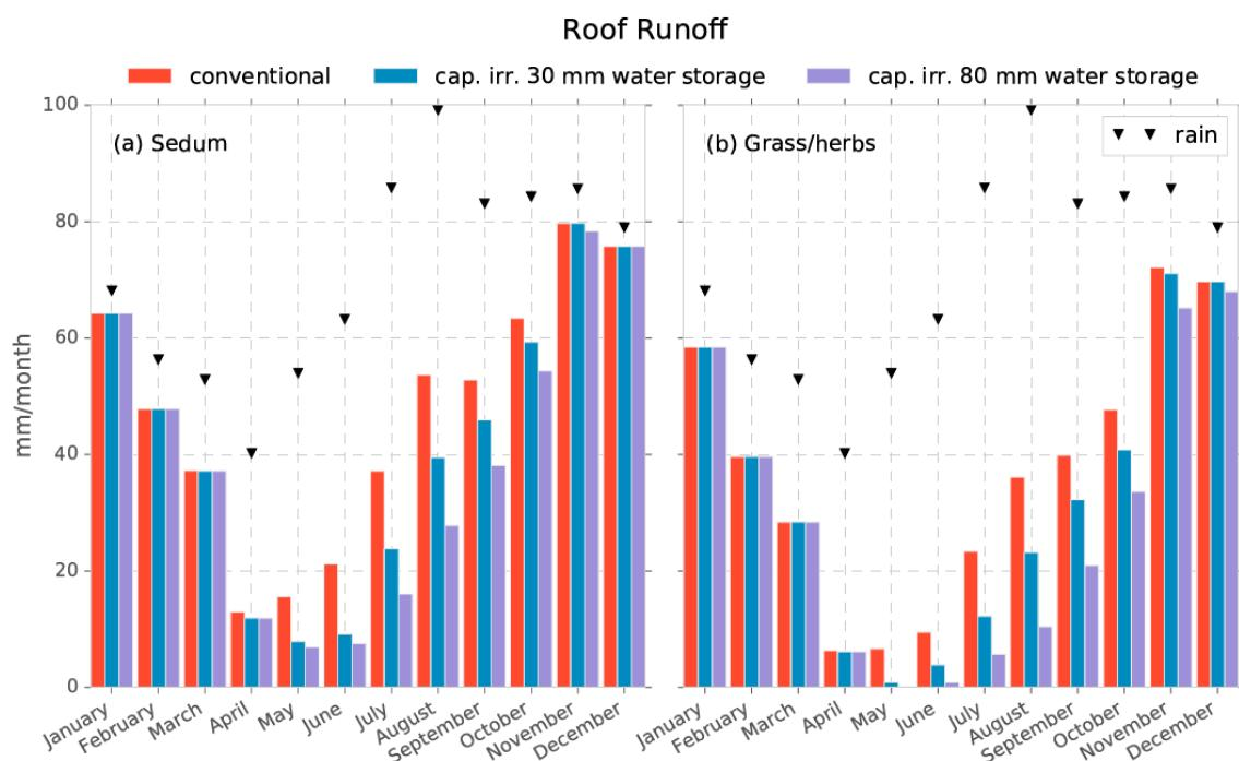
**Figure 11.** Estimated (with the bucket model) monthly averaged runoff for the six roof setups based on 30 years of Schiphol meteorological data. Black triangles denote the monthly averaged precipitation over the period 1988–2017.
