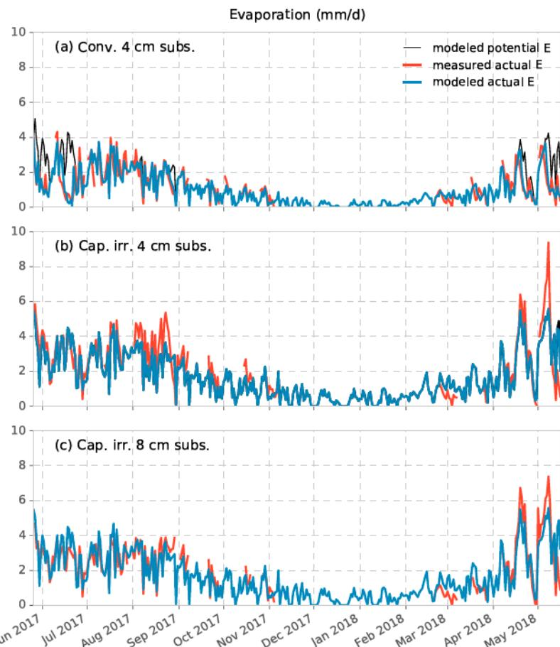
**Figure 5.** Measured and modeled daily evaporation for the three lysimeters. With  $E_p$  calculated with on-site measured variables (black line),  $E_a$  measured with weighing lysimeters (red line) and  $E_a$  modeled with the simple bucket model (blue line).
