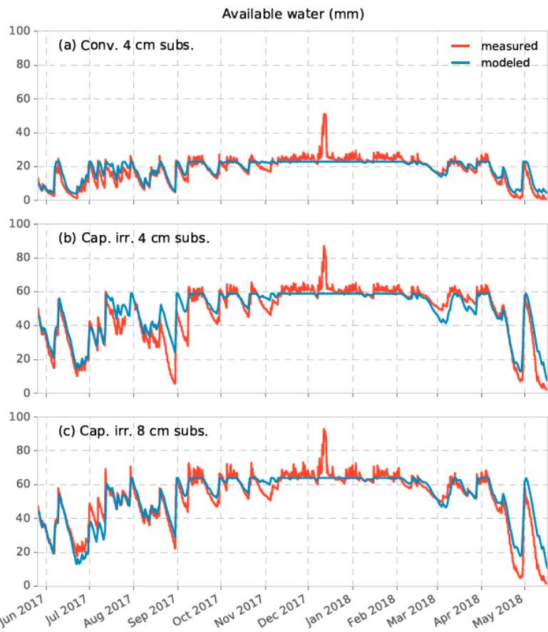
**Figure 7.** Measured and modeled daily water availability during the measurement period. Water availability was measured by subtracting the dead weight of the lysimeters from the total weight of the lysimeters over time. The measured peak in available water on 10 December 2017 is related to a heavy snowfall event that resulted in a strong increase of the lysimeter weight.
