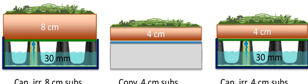
**Figure 2.** Schematic cross-sections of the three research plots. The left and right plot are equipped with the Permavoid drainage and capillary irrigation system.
