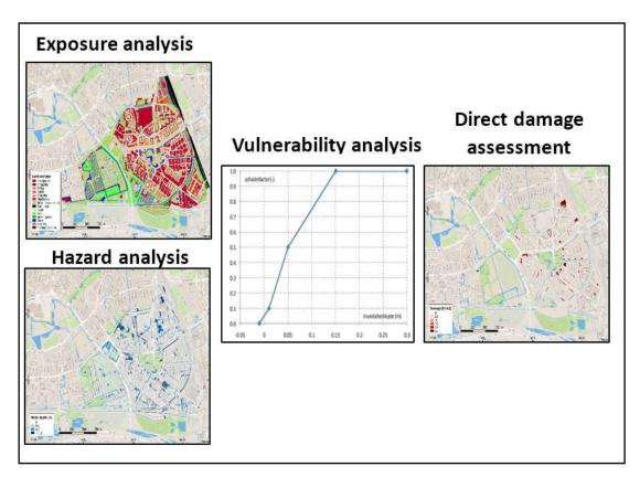
Figure 2. Standard direct flood damage assessment framework.
