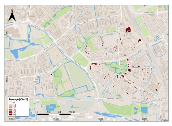
Figure 11. Lombardijen flood damage map (dark red signifies high flood damage).
