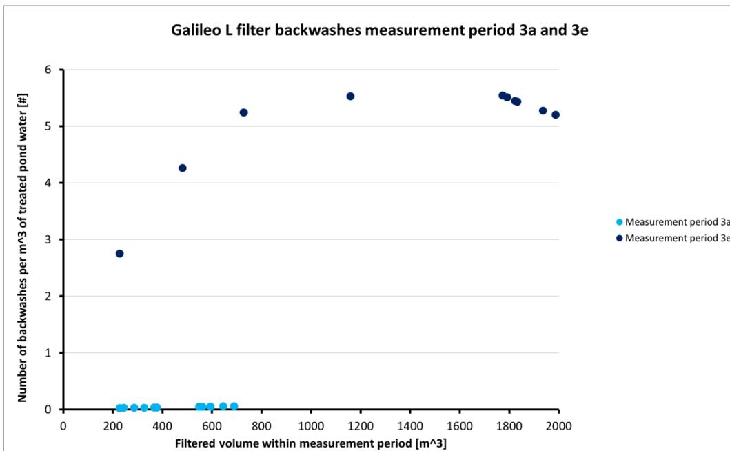
**Figure 4-18: Backwash frequency of the Galileo L filter during measurement periods 3a and 3e**
