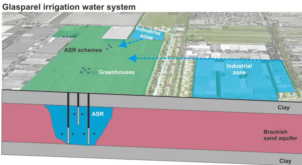
**Figure 2-2: Water system Glasparel+: an example of storm water harvesting, storage, and usage in modern greenhouse areas**
