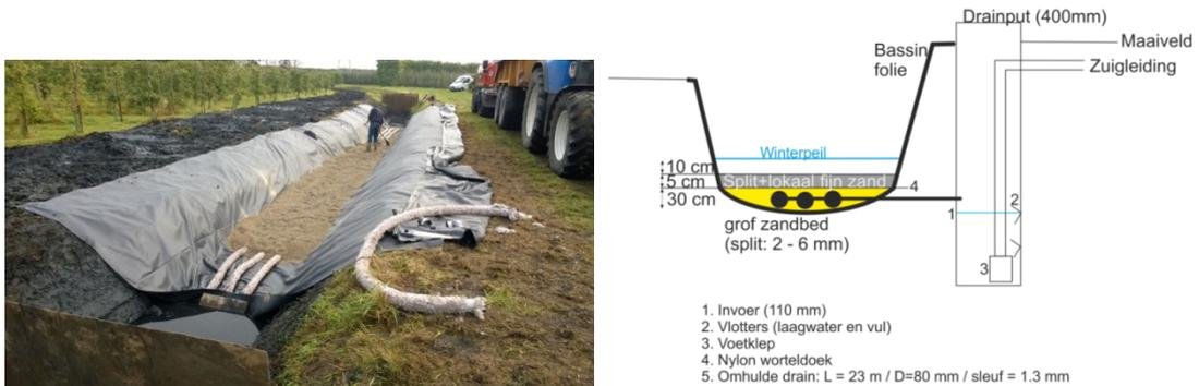
**Figure 3-11: Bottom filter at Freshmaker Ovezande (runoff ditch water)**
