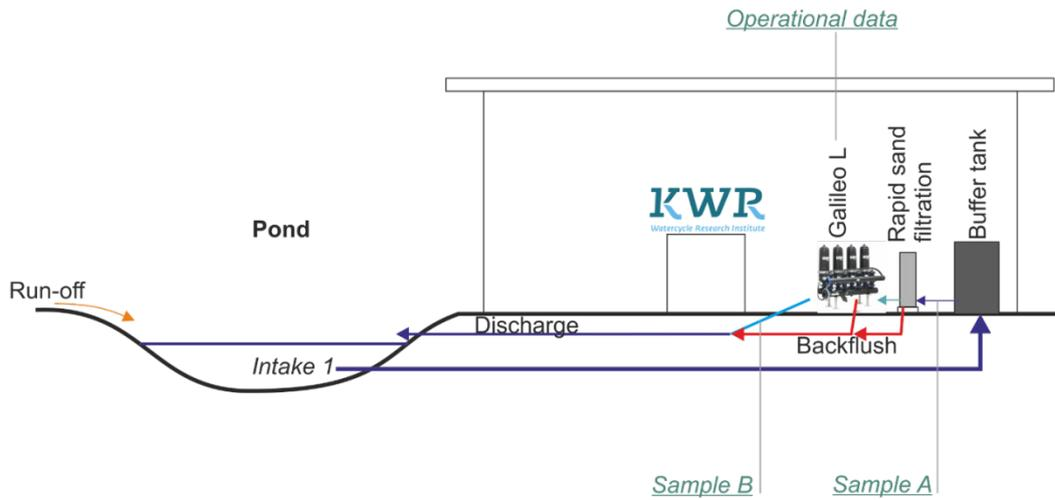
**Figure 4-8: Schematic overview of the complete set-up with the Galileo filter**
