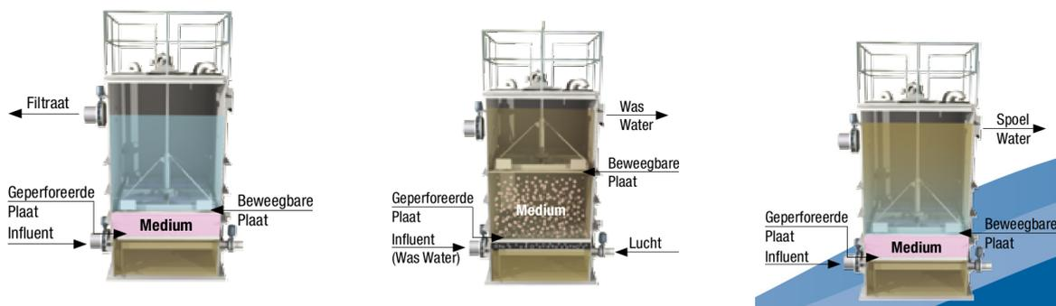
Figure 3-4: Operation of the Fuzzy filter (Bosman water management B.V.)
