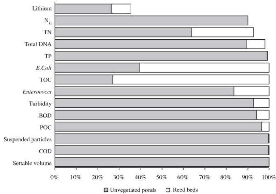
**Figure 3-10: Reduction of various parameters in buffer basins without vegetation and downstream (horizontal flow) reed beds after collection of sewage water in Grou, Friesland (the Netherlands) (Mulling et al., 2013). Note: potential impact of aging on removal efficiency not taken into account.**
