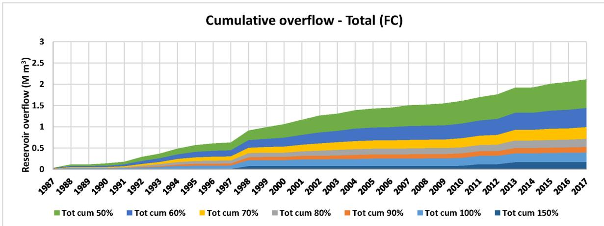
**Figure 2-10: Cumulative overflow considering forecasts (FC) during operation from January 1987 – December 2017. Well capacities are varied from 50% - 150% of the original (real) well capacities**
