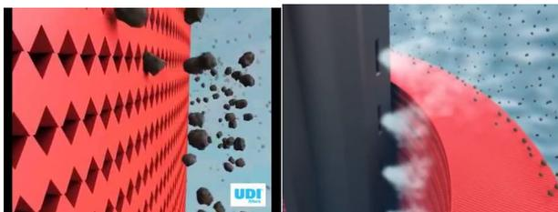
Figure 4-4: Illustration of filtration mechanism (left) and air/water flushing (right) of Galileo filter
