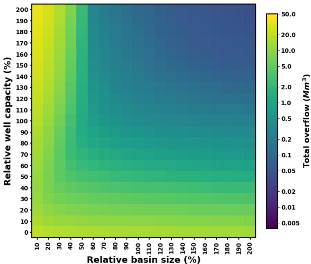
Figure 8-5: Cumulative total overflow from the owners' reservoirs and the storm water canals (in  $Mm^3$ ) with the reactive management approach (BAU) under various design conditions of relative well capacity and reservoir capacity. Model period: January 1987 – December 2017
