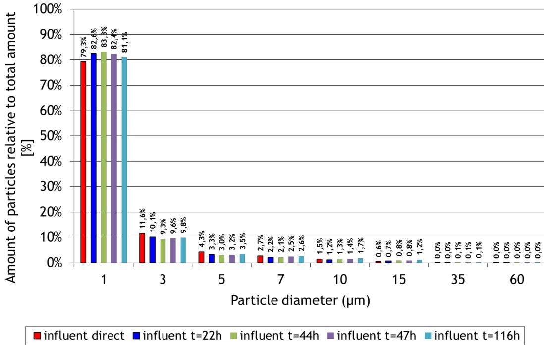
Figure 8-2: Relative amount of particles with respect to the total amount of particles measured in feed water
