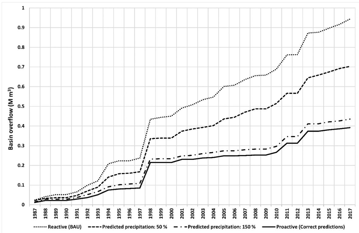
Figure 17: Cumulative overflow assuming either 100% correct predictions, or with an over- or underestimation by 50%; all compared to expected overflow with a reactive management approach.
