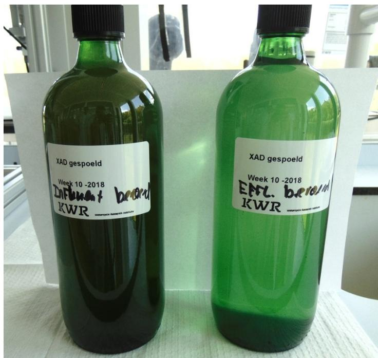
Figure 4-32: Sample of feed (left) and product (right) taken from the Galileo L filter during abnormal conditions
