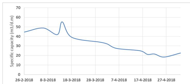
**Figure 4-26: Specific injection capacity of the infiltration well fed with Galileo L filter product in the period of 26-2-2018 to 3-5-2018. Not corrected for temperature.**
