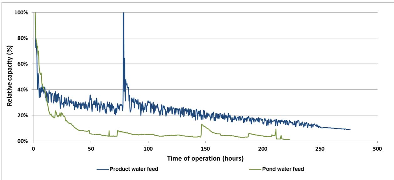
**Figure 4-20:** Capacity versus head relative to the initial (saturated) well capacity (in%) for the Feed and Product column. The Feed column experiment was done from 11 July 2017 until 20 July 2017. The Product column experiment was done from 24 July 2017 until 8 August 2017.
