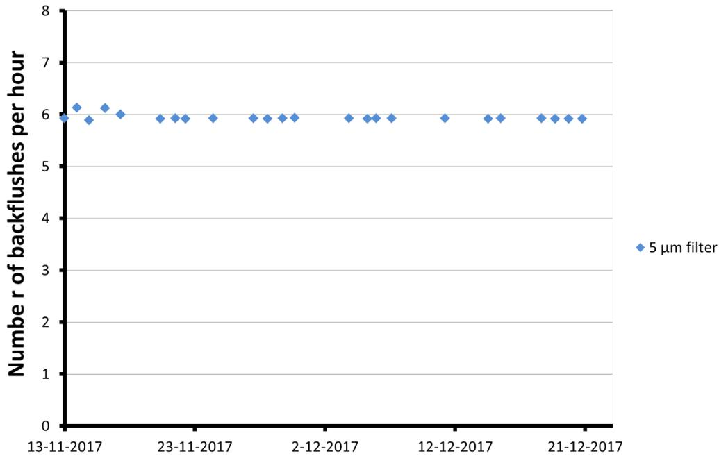
Figure 4-22: Number of back-flushes of Galileo L filter during test period (13-11 2017 till 21-12-2017)
