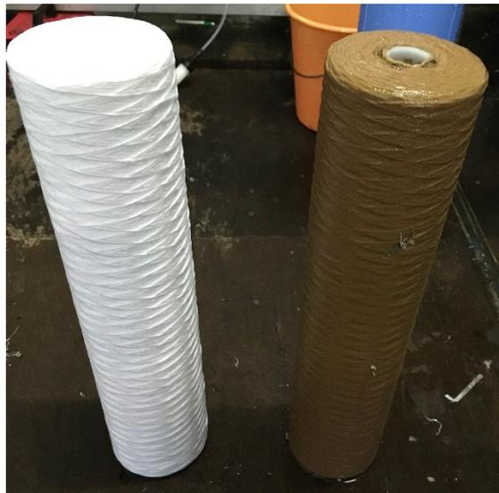
Figure 5-6: Fresh (left) and fouled (right) spun-wound 1 micron cartridge filter. Picture taken on 21-1-2019
