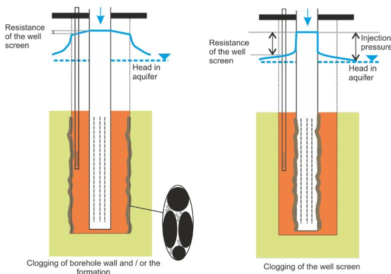
**Figure 3-2: Typical well clogging due to particles**
