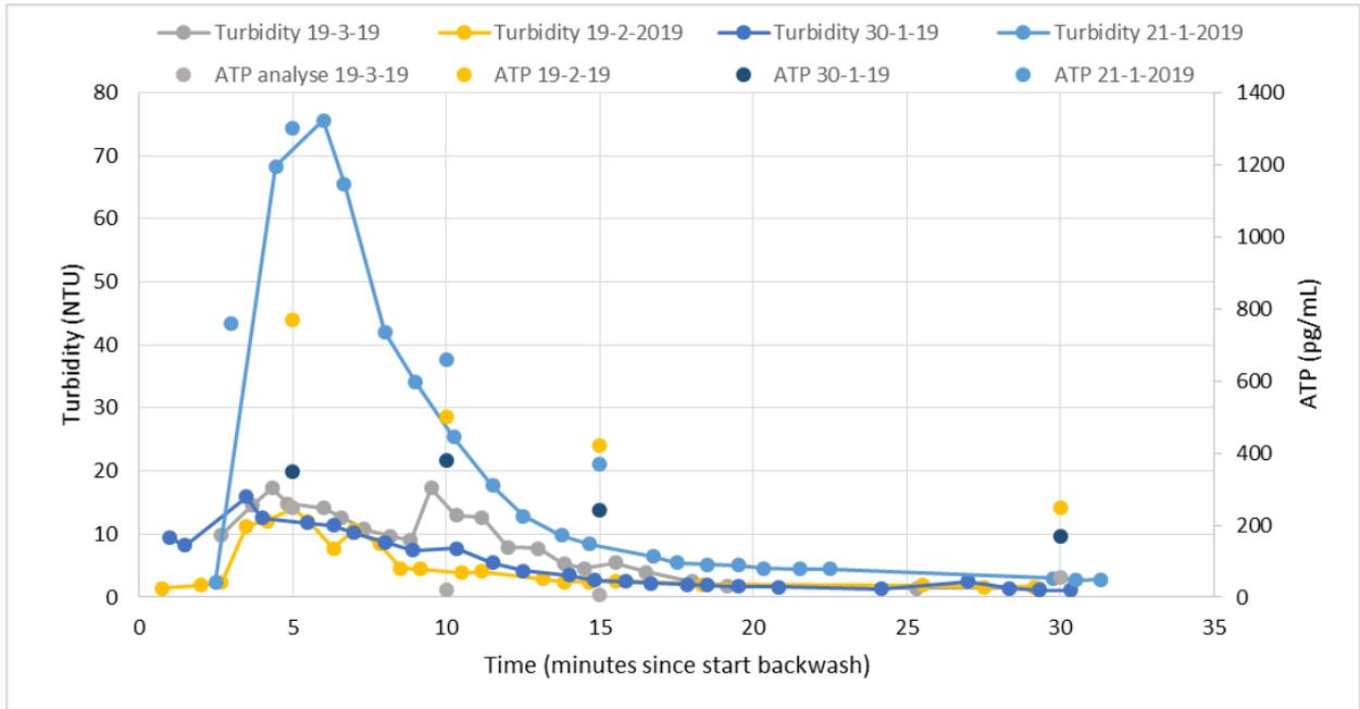
Figure 5-5: Observed turbidity and ATP during backwash of the well
