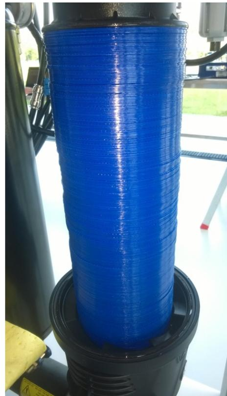
Figure 4-5: Compressed 50 micron filter discs on the Galileo L filter
