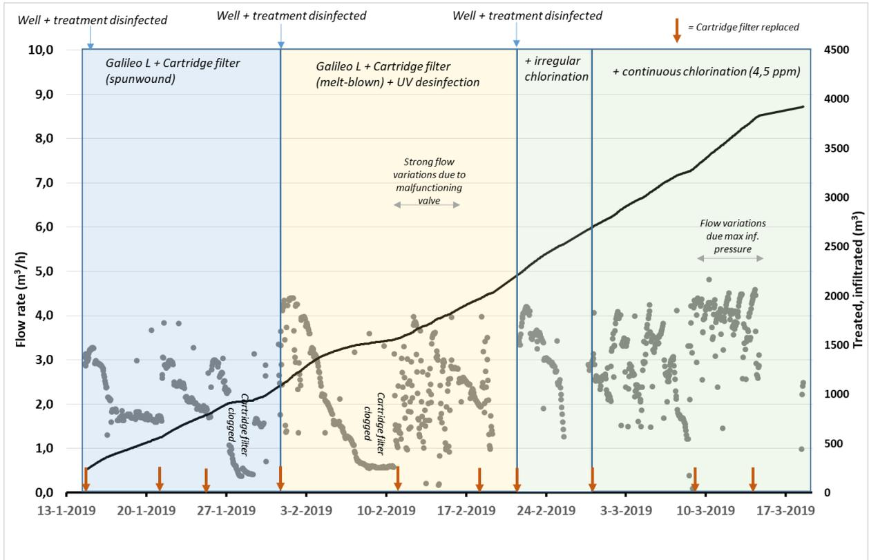
Figure 5-1: Measured flow rate and cumulative infiltration volume during 2019 trial. Black line = treated, infiltrated water. Grey dots refer to infiltration flow rate.
