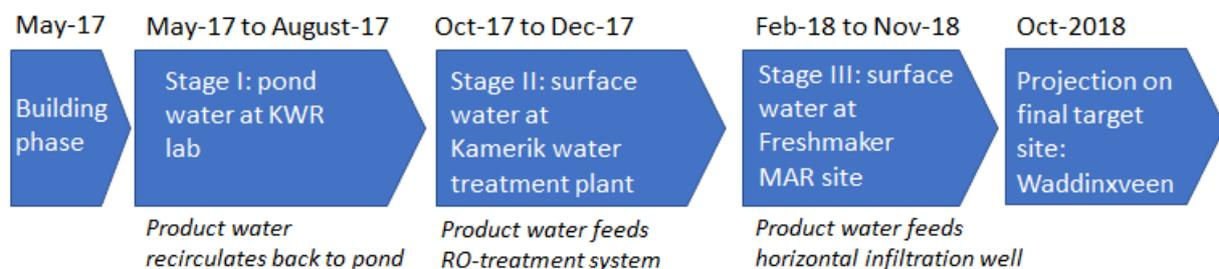
**Figure 4-2: Stepwise approach to test the Galileo L filtration system**
