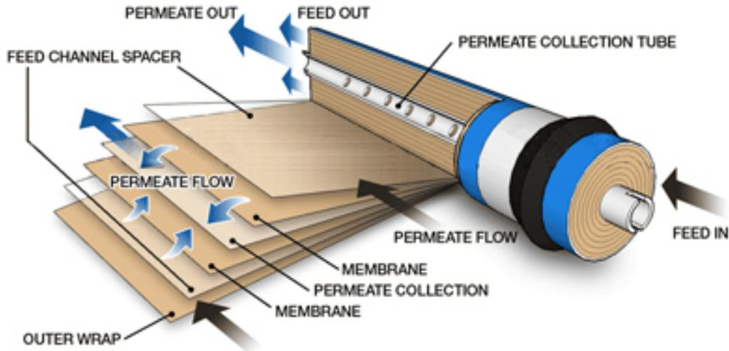
Figure 4-11: Schematic overview of a reverse osmosis membrane
