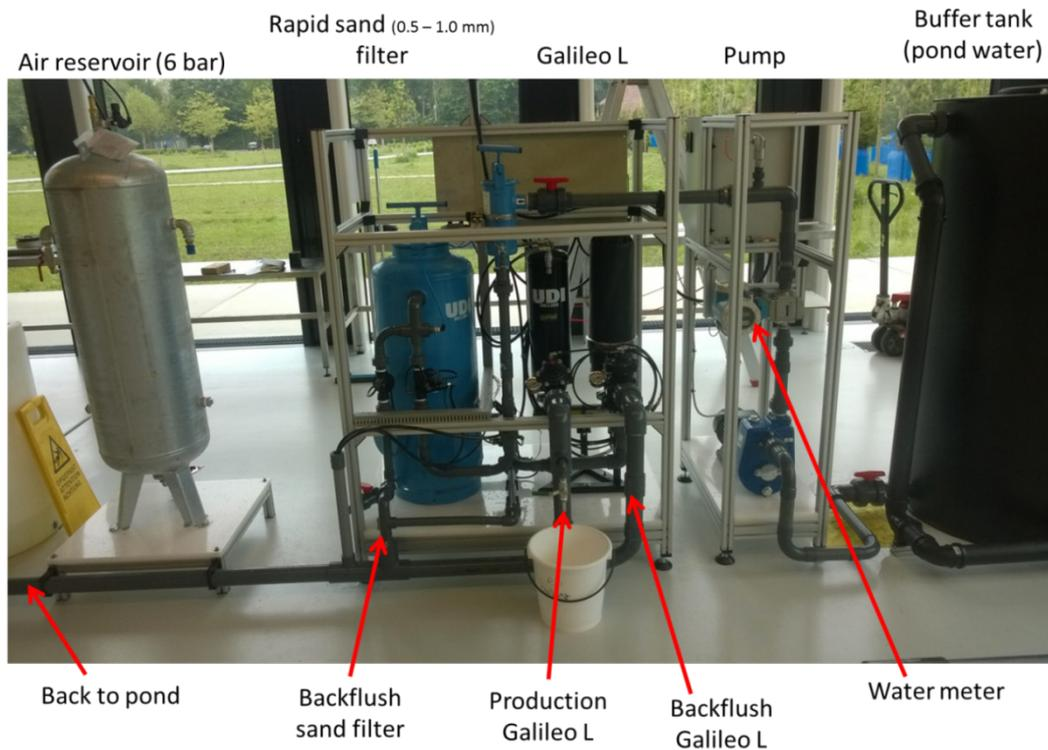
**Figure 4-9: Set-up of the filtration experiment in the KWR laboratory**
