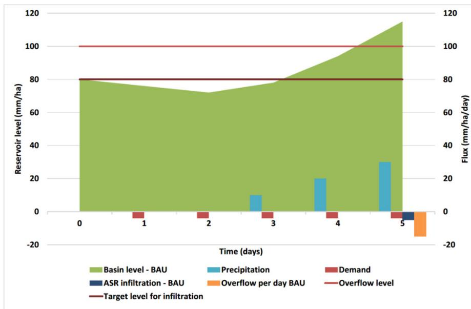
**Figure 2-5: Reactive management approach: ASR infiltration only when reservoir level exceeds target level for infiltration. The overflow event is only slightly reduced. BAU = business as usual (standard, current way of operation)**
