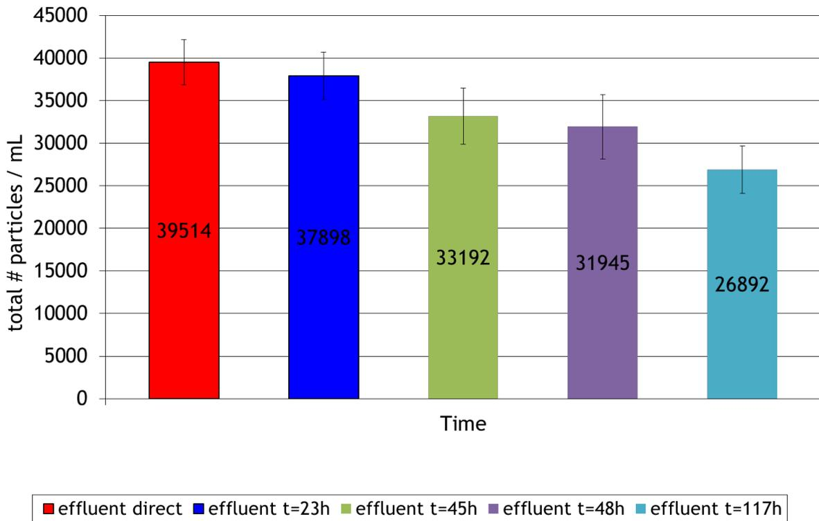
Figure 8-3: Total amount of particles in product water over time
