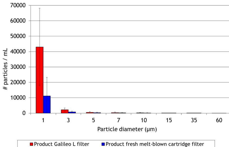
Figure 5-11: Particle counting results of a fresh melt-blown filter on January 30.
