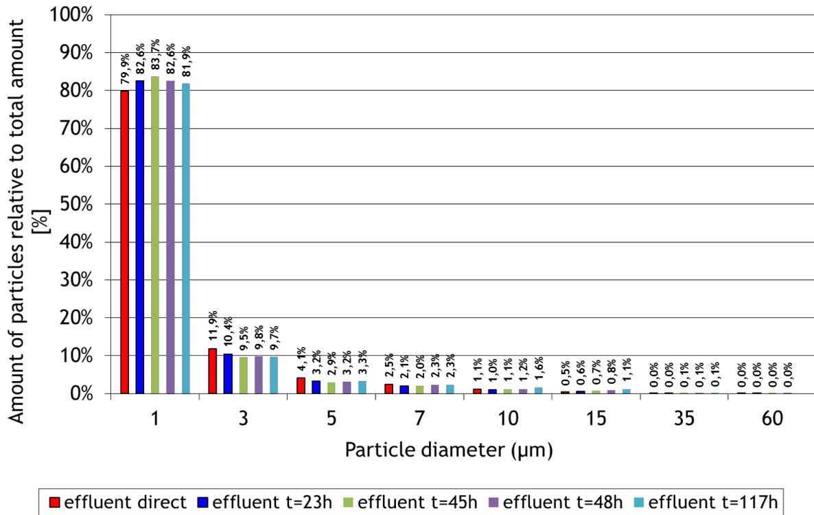
Figure 8-4: Relative amount of particles with respect to the total amount of particles measured in product water
