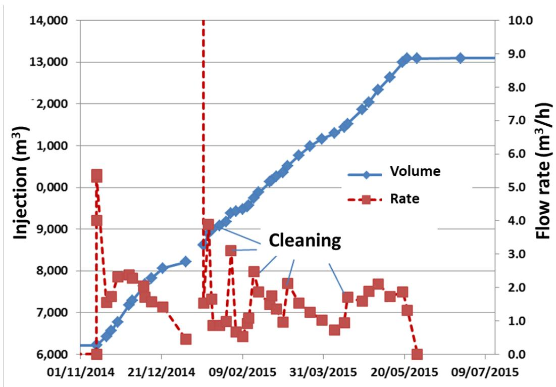
Figure 3-13: Development of the flow rate from canal bed filtration unit in Ovezande in 2014/2015. Injectie = injection, debiet = capacity, schoonvegen toplaag = cleaning.
