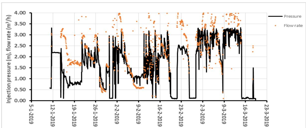
Figure 5-2: Observed pressure on the infiltration well. No correction was made for temperature (varying between 4-10 °C).
