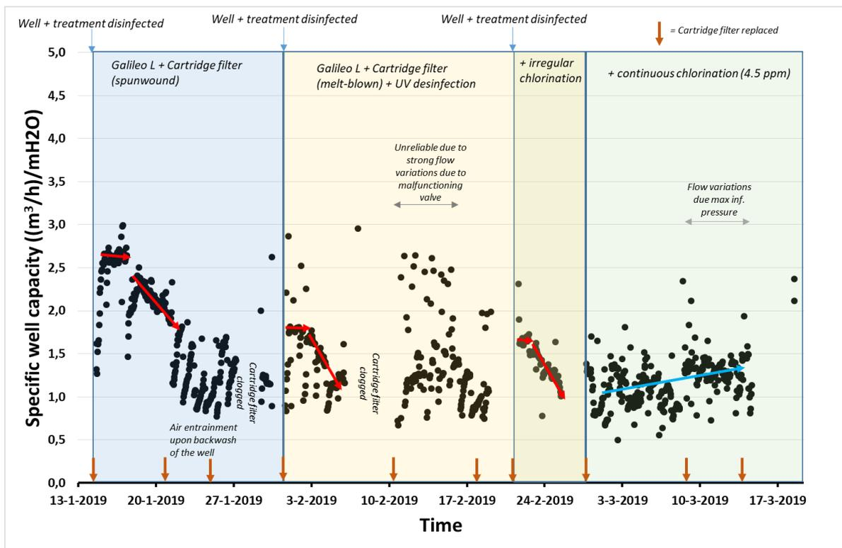
Figure 5-13: Specific capacity of the infiltration well in 2019.
