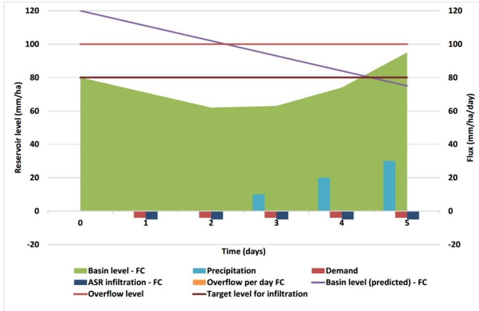
**Figure 2-6: Proactive management approach: ASR infiltration when predicted reservoir level exceeds target level for infiltration. The actual reservoir level is lowered before the precipitation is actually occurring. FC = forecasting based (new way of operating based on predictions of rainfall and water use)**
