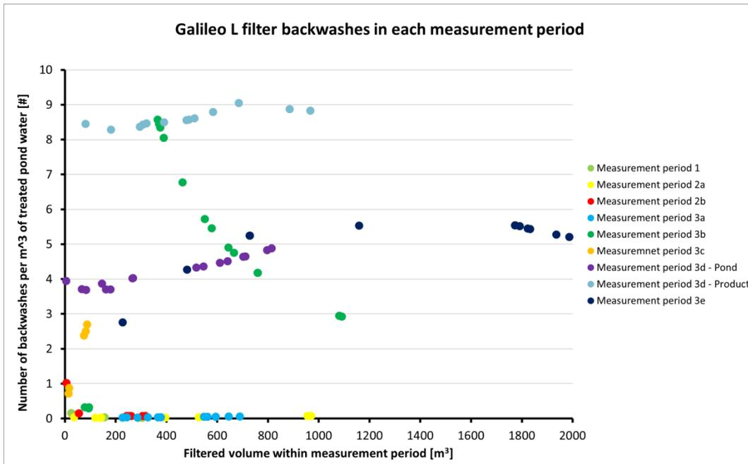
**Figure 4-17: Backwash frequency of the Galileo L filter during individual measurement periods**
