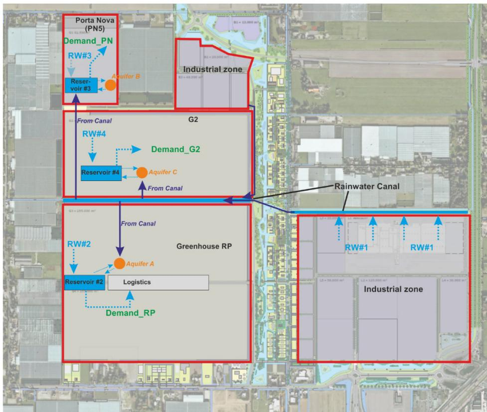
Figure 2-3: Top view of the Glasparel+ water system including water fluxes
