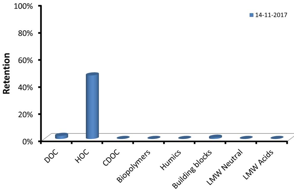
Figure 4-23: Retention of various organic compounds by the Galileo L filter
