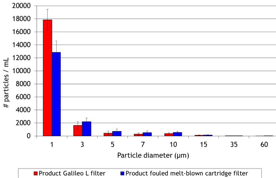
**Figure 5-12: Particle counting results of a fouled melt-blown filter on February 19.**
