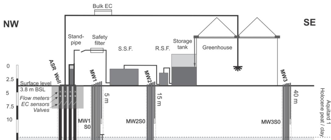
**Figure 3-3: Application of slow and rapid sand filtration in ASR in horticulture (The Netherlands), especially for removal of suspended solids (K. G. Zuurbier, Zaadnoordijk, & Stuyfzand, 2014). R.S.F. = rapid sand filter, S.S.F. = slow sand filter)**
