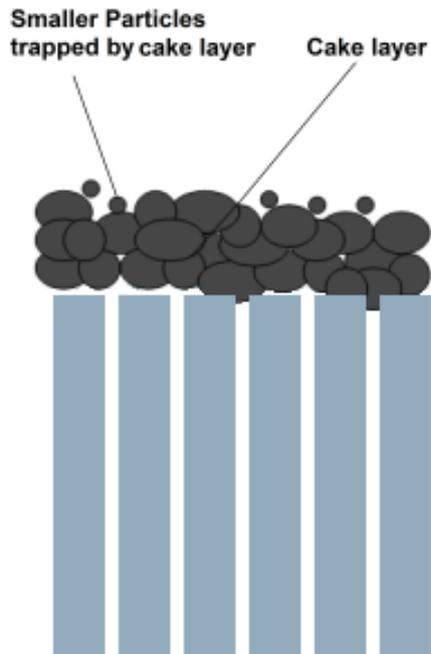
Figure 4-31: Systematic overview of cake layer development. as big particles block the filter channels, particles having a diameter smaller than the filter mesh size can be blocked by these bigger particles forming a dense layer
