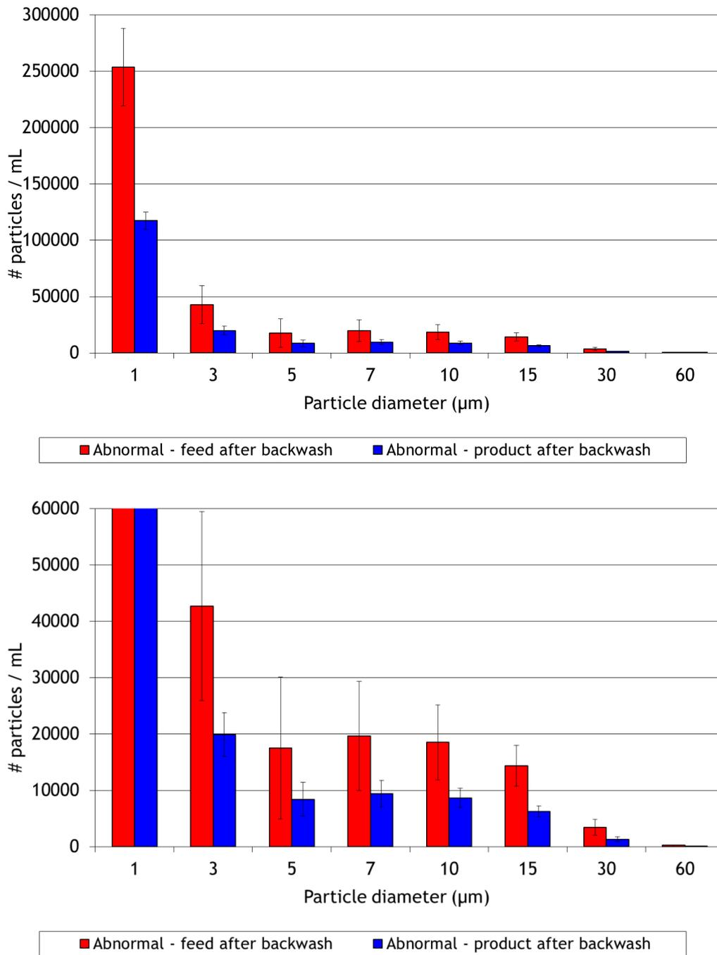
Figure 4-37: Measured amount of particles in the feed and product water of the Galileo L filter during abnormal conditions just after a backwash (19-6-2018): with a low resolution (top), and in more detail (bottom).
