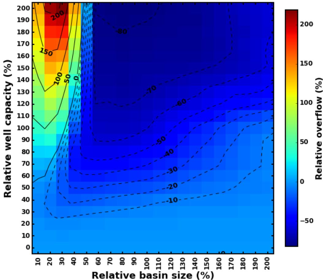
Figure 2-16: Relative increase (+) or decrease (-) in overflow with proactive instead of reactive reservoir management as a result of changing either/or the well capacity and reservoir size of the system relative to the real situation (at 100%).
