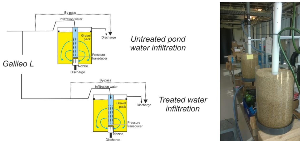
**Figure 4-10: Schematic overview of the model infiltration test well (left) and two scale model infiltration wells for evaluation of the clogging potential (right)**
