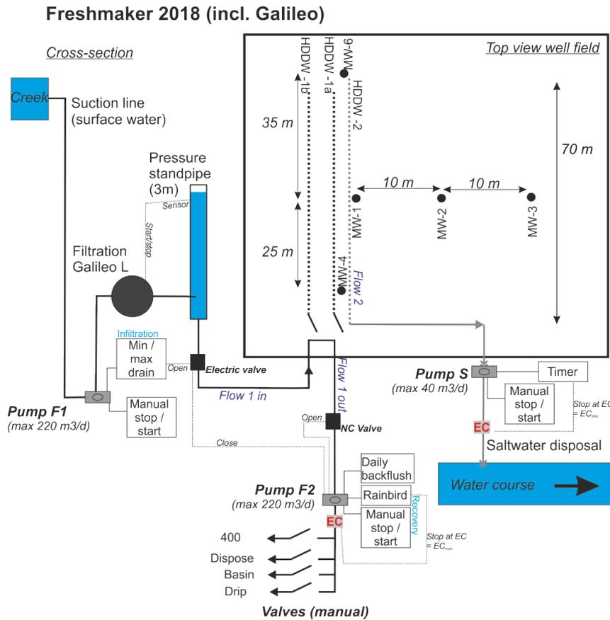
Figure 4-15: Flow scheme at the Freshmaker site after incorporation of the Freshmaker
