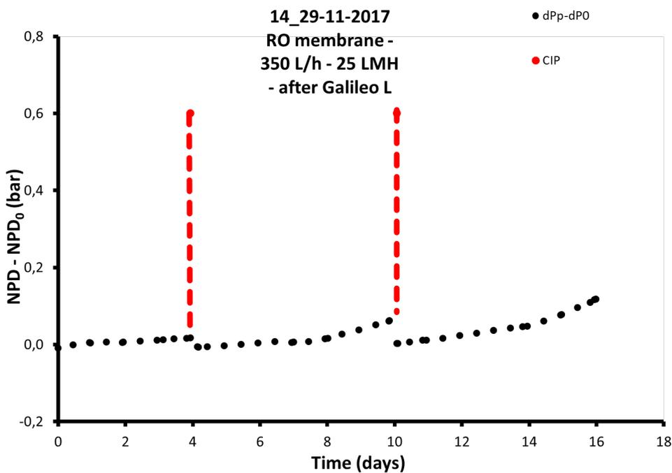
Figure 4-24: Normalized pressure drop of RO membrane fed with Galileo L product water. The two red lines indicate clean in place (CIP) procedures in which the RO membrane is chemically cleaned
