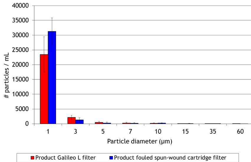
**Figure 5-8: Particle counting results of a (very) fouled spun-wound filter on January 21.**
