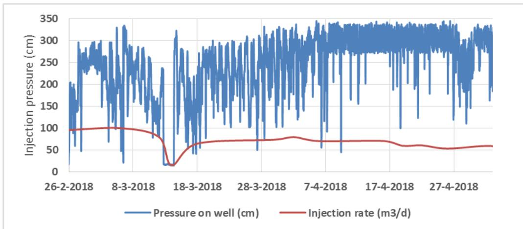
**Figure 4-25: Pressure on infiltration well (blue line) and injection rate (red line) in the period 26-2-2018 to 3-5-2018. Sharp variations in injection pressure are caused by regular infiltration well backwash. From 12-3-2018 till 14-3-2018 the installation was stopped due to clogging of the feed water intake**
