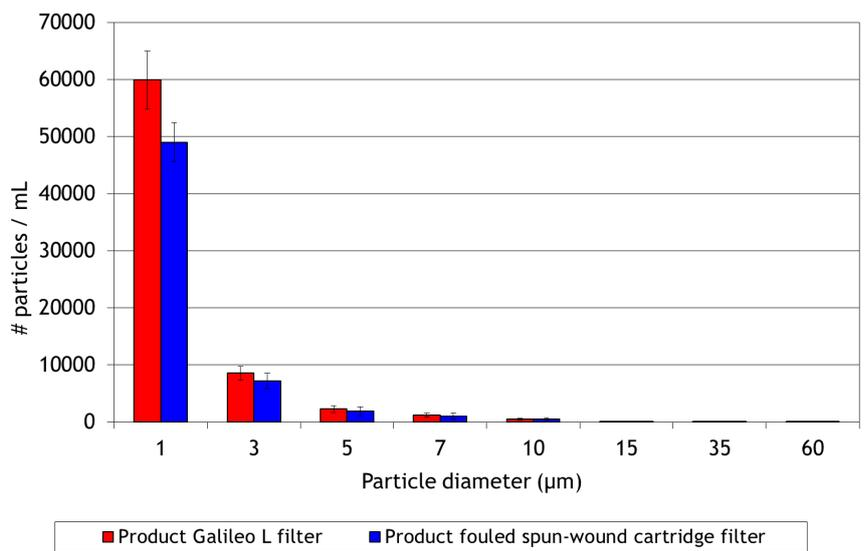
**Figure 5-7: Particle counting results of a fouled spun-wound filter on January 17.**
