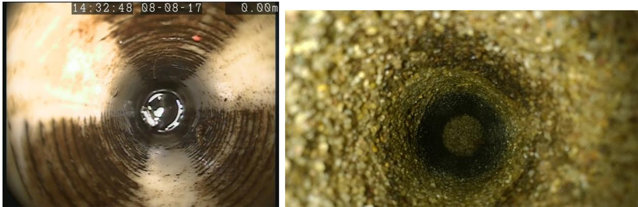
**Figure 4-21: Camera inspection result of the well infiltrating the Galileo product water. before (left) and after (right) removing the well screen.**
