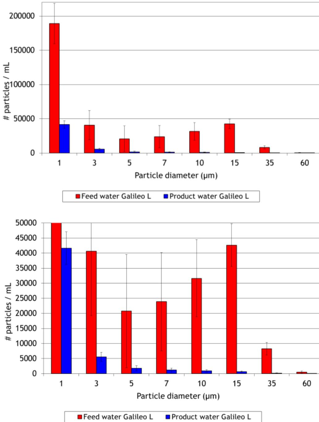
Figure 4-30: Measured amount of particles in the feed and product water of the Galileo L filter during abnormal conditions (May 3, 2018): with a low resolution (top), and in more detail (bottom).
