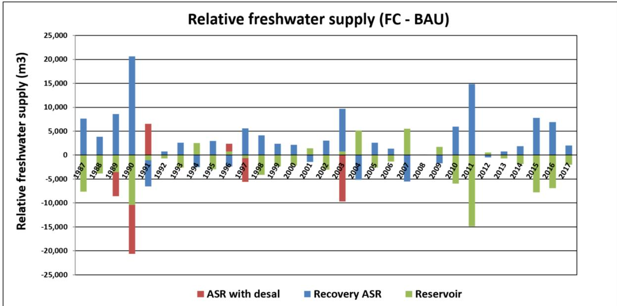
**Figure 2-15: Difference in the type of freshwater supply source (FC – BAU: proactive minus reactive): precipitation without infiltration (“Reservoir”), directly usable after recovery (“Recovery ASR”) or after recovery with desalination (“ASR with desal”)**
