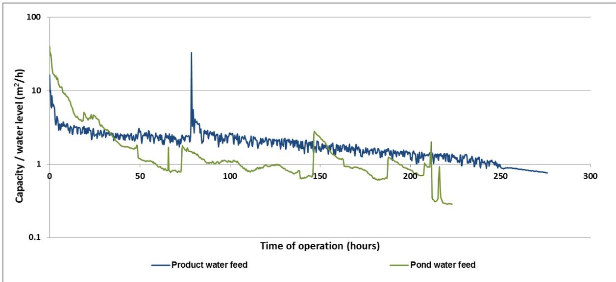
**Figure 4-19:** Well capacity divided by the water level (m<sup>3</sup>/h/m or m<sup>2</sup>/h) in the Feed and Product columns over time. The Feed column experiment was done from 11 July 2017 until 20 July 2017. the Product column experiment was done from 24 July 2017 until 8 August 2017
