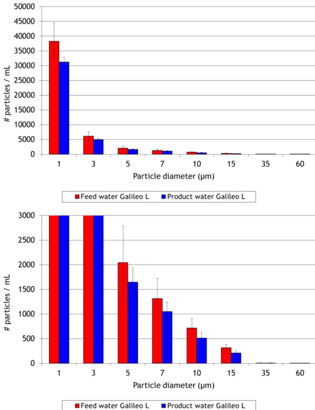
Figure 4-28: Measured distribution of particles in feed (red) and product (blue) water of the Galileo L filter during normal conditions: with a low resolution (top), and in more detail (bottom).
