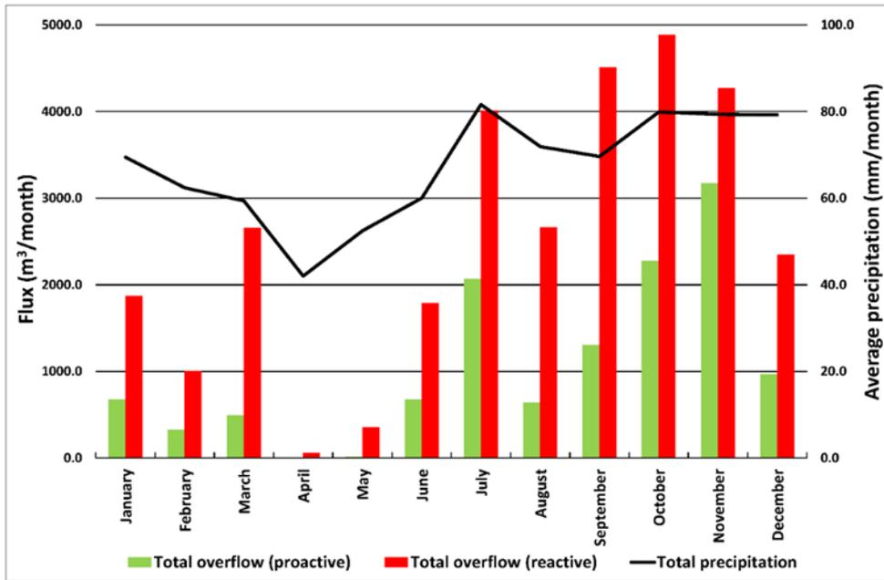
Figure 2-8: Average monthly overflow with the reactive and proactive management approach (in m<sup>3</sup>/month), and the average monthly precipitation (in mm).
