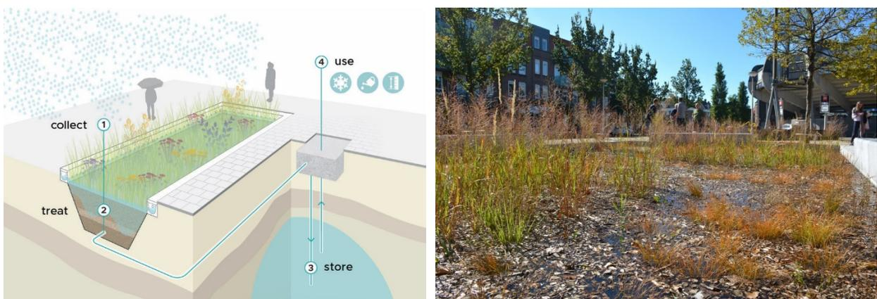
**Figure 3-8: Blue Bloqs, currently under development (left) and first pilot at Spangren, Rotterdam**
