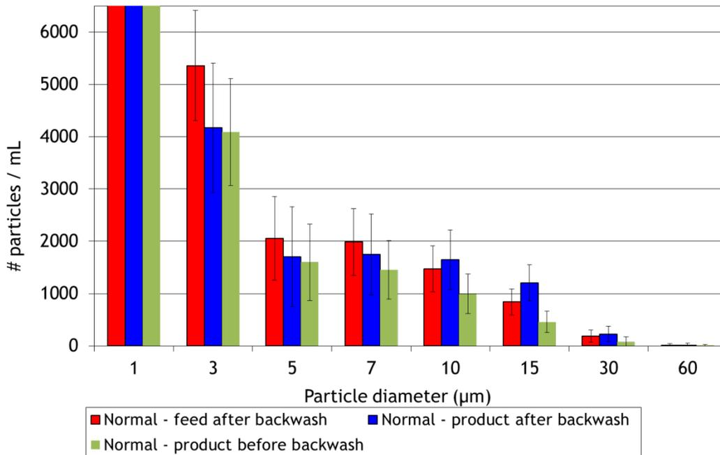
**Figure 4-35: Galileo L filter performance during normal conditions: with a low resolution (top), and in more detail (bottom). red = feed water, blue = product water after backwash, green = product water before backwash**
