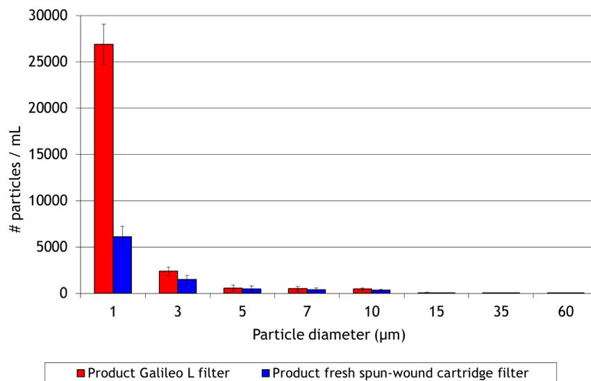
**Figure 5-9: Particle counting results of a fresh spun-wound filter on January 21.**
