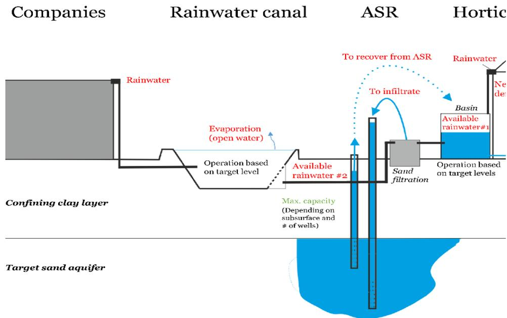
Figure 2-4: Schematic overview of the Glasparyl+ water system components including water fluxes
