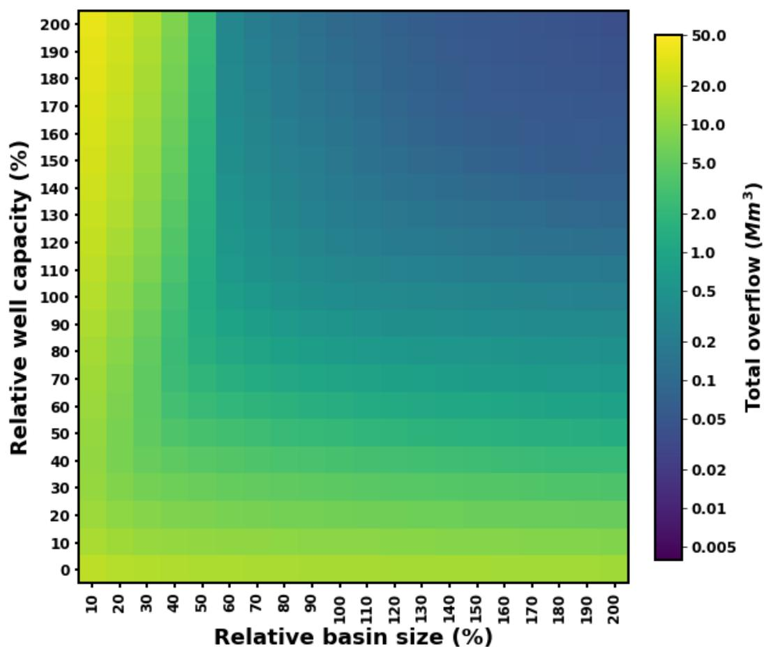
Figure 8-6: Cumulative total overflow from the owners' reservoirs and the storm water canals (in Mm<sup>3</sup>) with the proactive management approach under various design conditions of relative well capacity and reservoir capacity. Model period: January 1987 – December 2017
