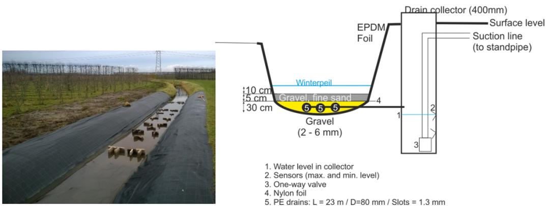
Figure 4-16: Current sand filter ('river bed filtration') at the Freshmaker site
