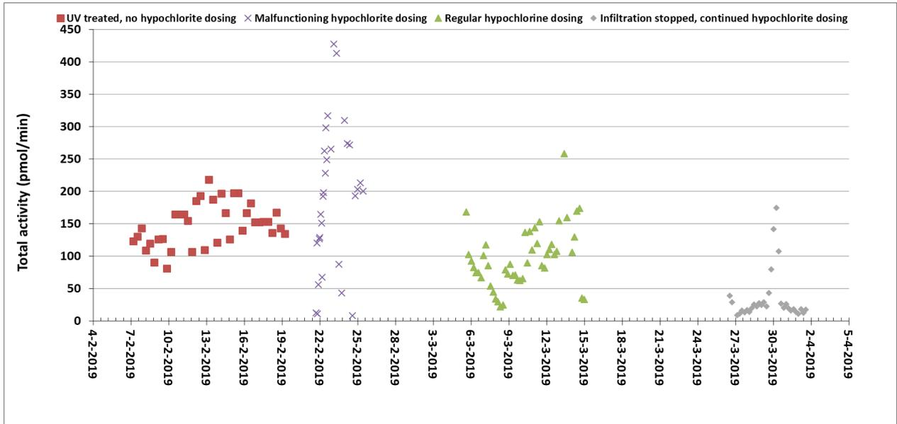
**Figure 5-4: Total activity measured in the water right before infiltration in the aquifer. Hypochlorite dosing causes the total activity to drop**
