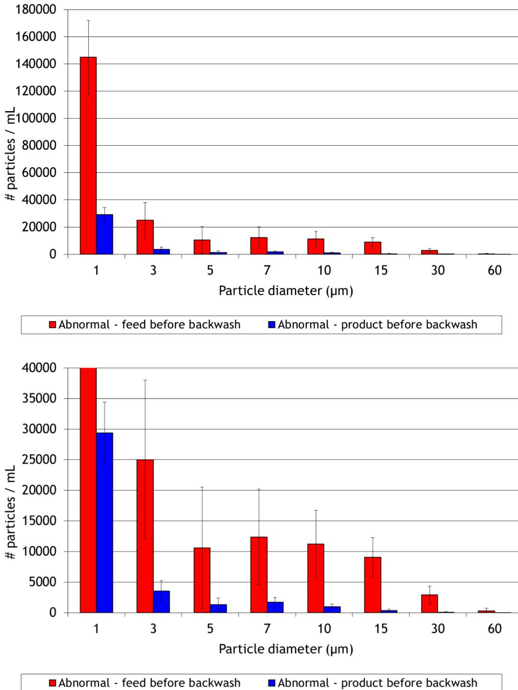
**Figure 4-36: Measured amount of particles in the feed and product water of the Galileo L filter during abnormal conditions just before a backwash (19-6-2018): with a low resolution (top), and in more detail (bottom).**
