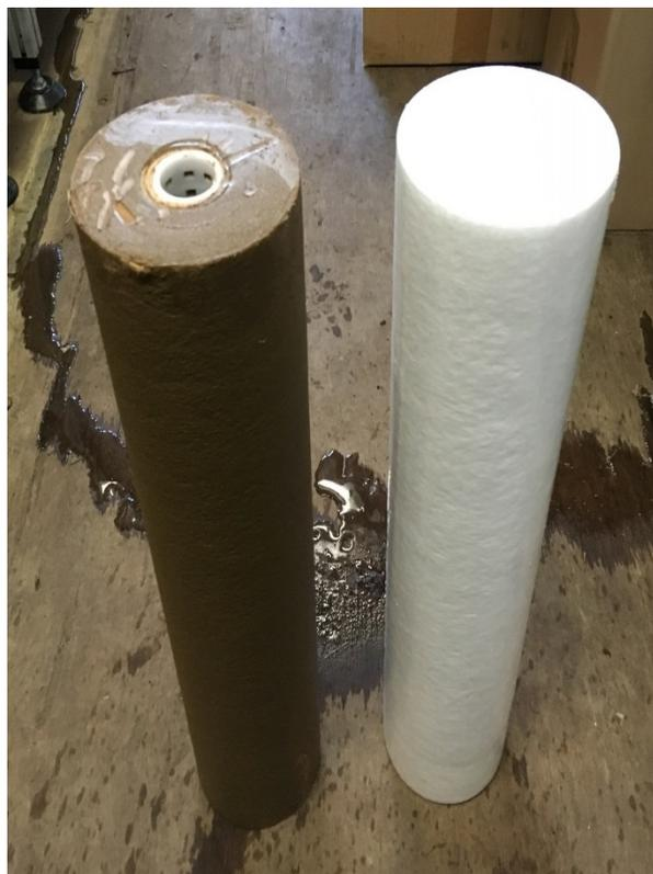
Figure 5-10: Fouled (left) and fresh (right) melt-blown 1 micron cartridge filter. Picture taken on 19-2-2019
