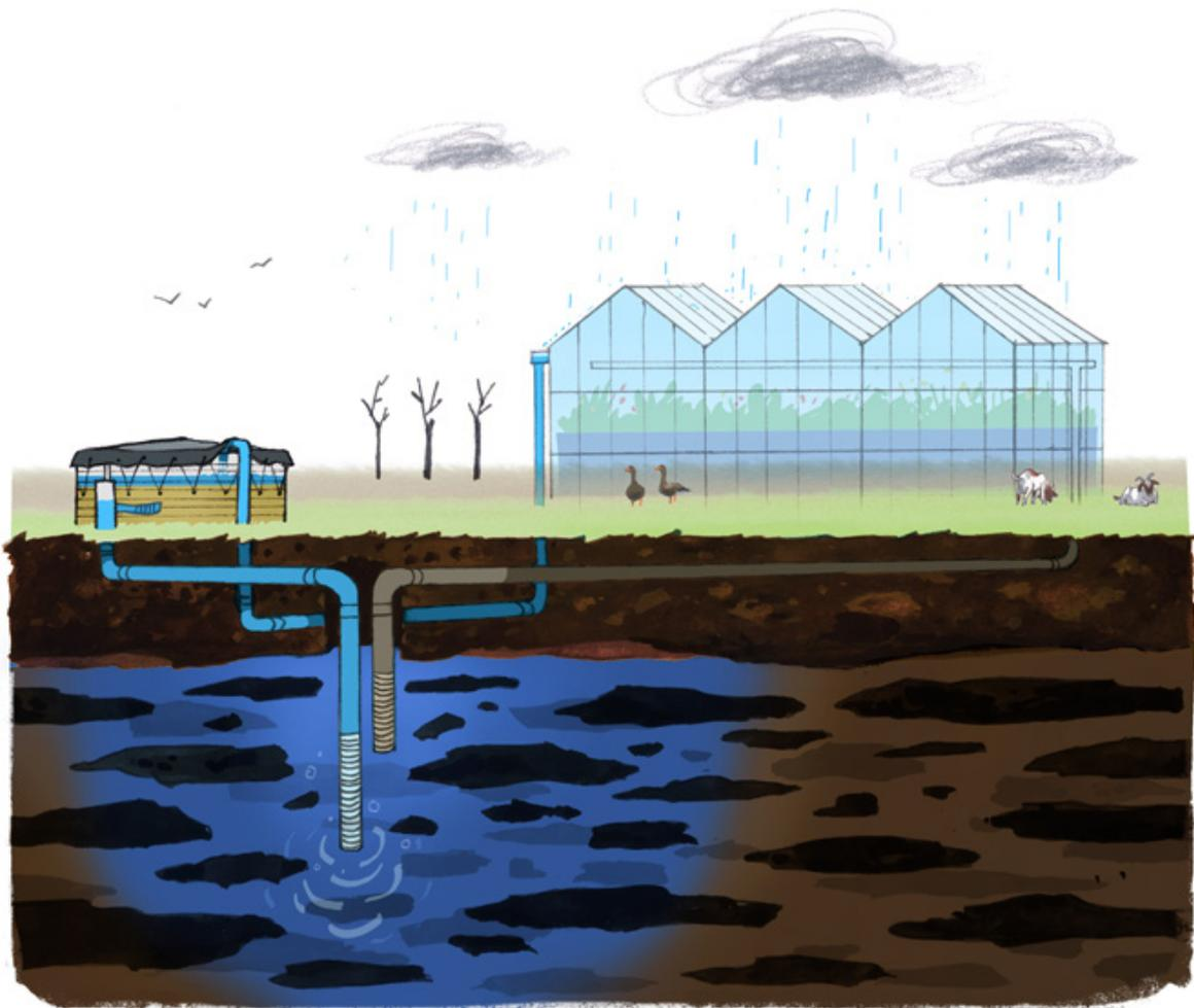
Figure 4-1: Impression ASR using slow sand filtration to treat storm water from greenhouse roofs
