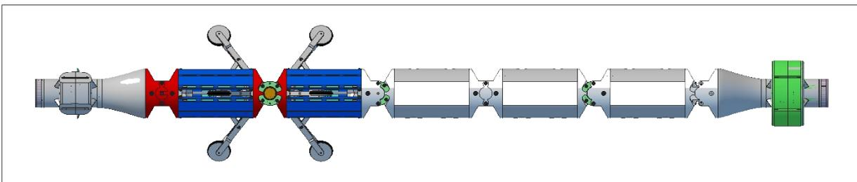
*Figure 2: CAD model representing the selected design concept. From the left to the right, the following modules are present: propulsion + vision, centering (2x), battery/electronics (3x), propulsion + vision.*
