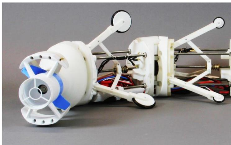
*Figure 3: Robot prototype. One propulsion + vision module and two clamping modules are shown.*
