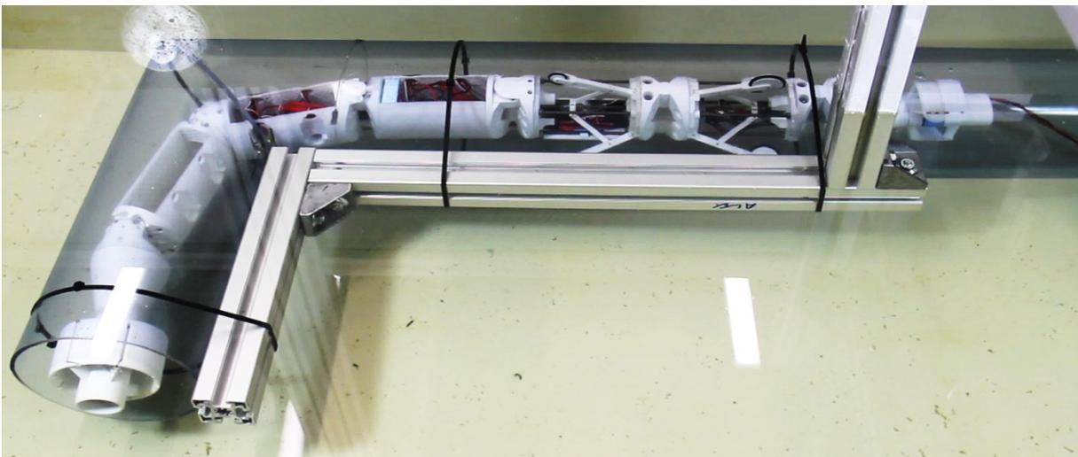
*Figure 4: Test passing a miter bend, using a 150mm I.D. pipe placed in a tank filled with water. The robot is self-centering and self-propelled, but is controlled manually by cable.*
