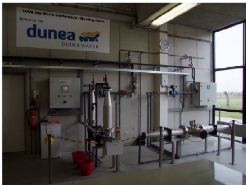
Figure 7-3 LP (on the left) and MP (on the right) pilot plant at Duena
