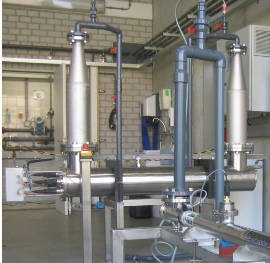
Figure VIV-1: LP pilot reactor at Dunea; on the left side the actual reactor, on the right side the schematic view
