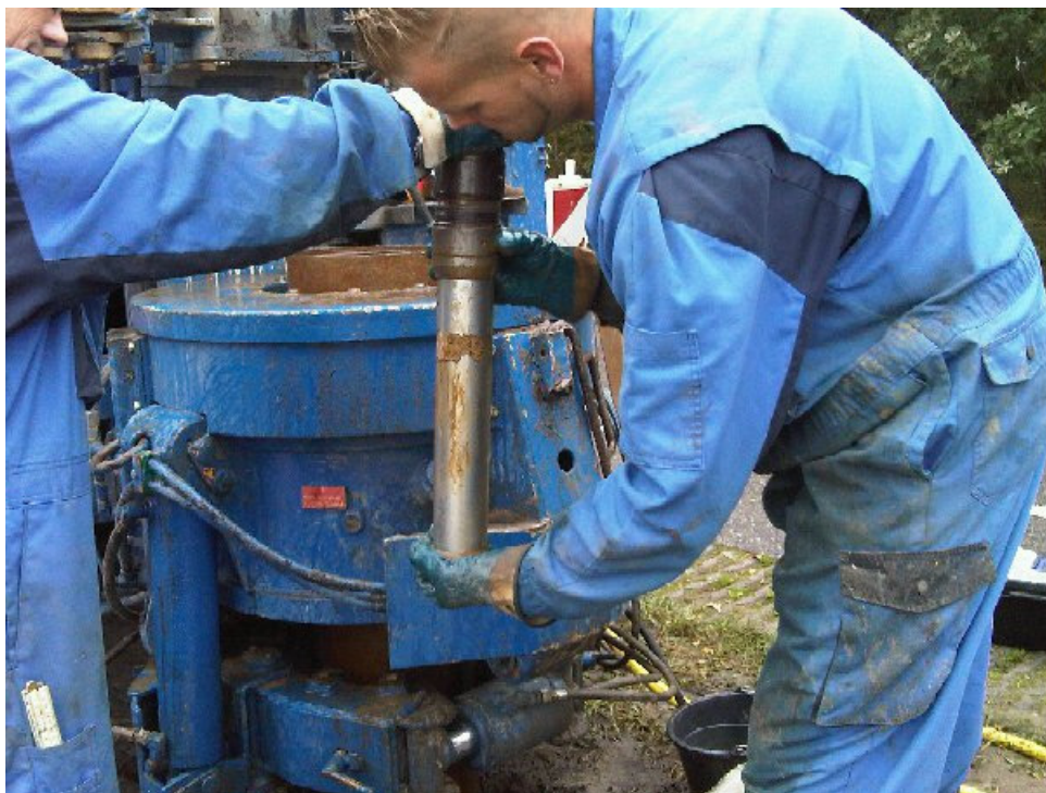
Collection of sediment core at Helvoirt
