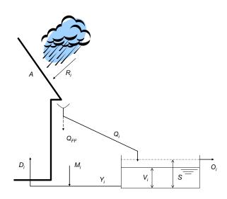
More detailed designs can be made with the so-called behavioural (stochastic) models. Ward *et al.* (2010b) show that these models lead to storage tanks that are substantially smaller than those based on simple mass balance simulations. The behavioural models simulate a (semi-) continuous mass balance from input (rainwater and suppletion), output (demand and overflow) and stored volume on a fixed time interval basis (Palla *et al.* 2011):
