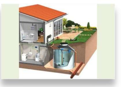
Figure 9: Example of a small scale individual RWH system.
