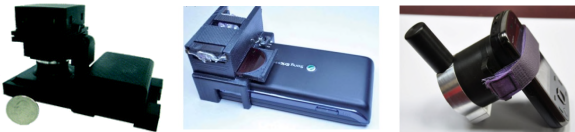
FIGURE 3: ADD-ON SMARTPHONE-BASED MEASUREMENT DEVICES FOR THE DETERMINATION OF MICROBIOLOGICAL PARAMETERS E. COLI , GIARDIA CYSTS AND DNA BY DETECTION OF FLUORESCENCE [52, 54, 57].
