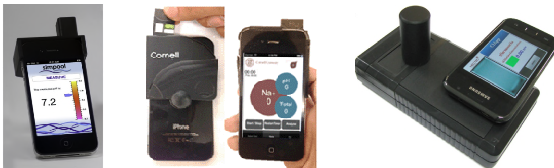
FIGURE 2: ADD-ON SMARTPHONE-BASED MEASUREMENT DEVICES FOR THE DETERMINATION OF PH AND CHLORINE-RESIDUE IN WATER BY COLORIMETRY [36-38].
