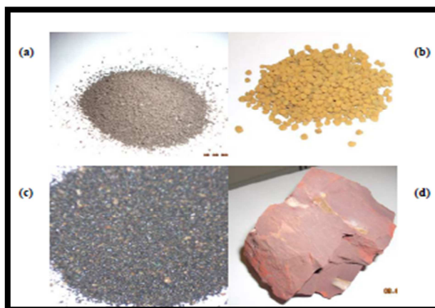
Figure 4.1: Different types of adsorptive media. a) Aquamandix b) IOCS c) Manganese greensand d) A stone of iron ore which can be crushed and pulverized (Buamah, 2009).
