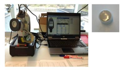
Figure 6. Handheld XRF analyser (left) and soil samples (right)
