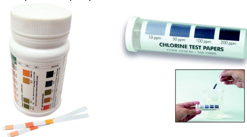
Figure 3-1 Examples of test strips for pH and chlorine
