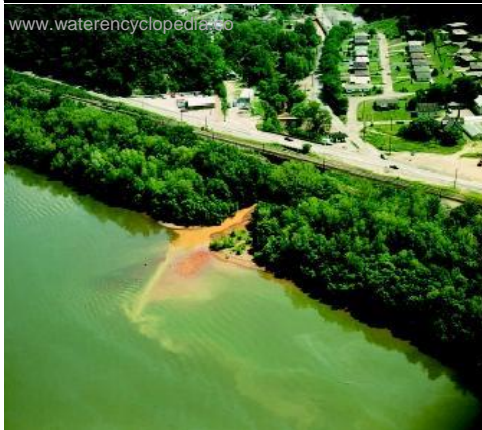
Figure 3-1 Example of variation in water quality sampling due to mixing conditions at a discharge
