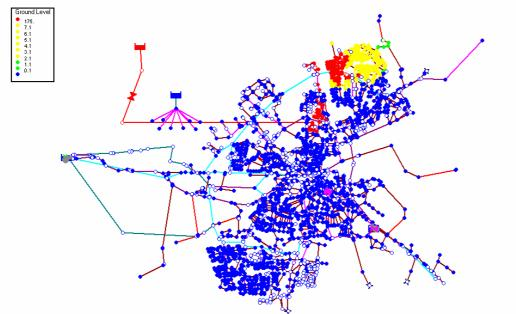
**Figure 2.8:** Calculated maximum concentrations when introducing a contaminant in a distribution pipe on the northern edge of the distribution area, reporting interval 30 minutes. The legend heading ground level should be replaced by concentration.
