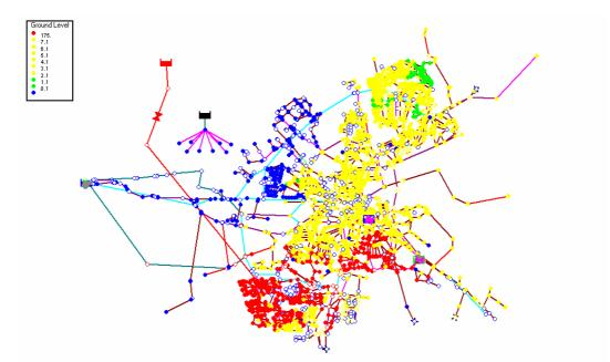
**Figure 2.7:** Calculated maximum concentrations when introducing a contaminant in a distribution pipe on the southern edge of the distribution area, reporting interval 30 minutes. The legend heading ground level should be replaced by concentration.
