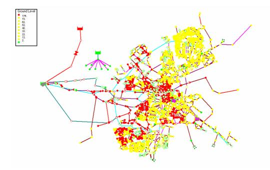
**Figure 2.5:** Calculated maximum concentrations when introducing a contaminant at the pumping station, reporting interval 10 minutes. The legend heading ground level should be replaced by concentration.
