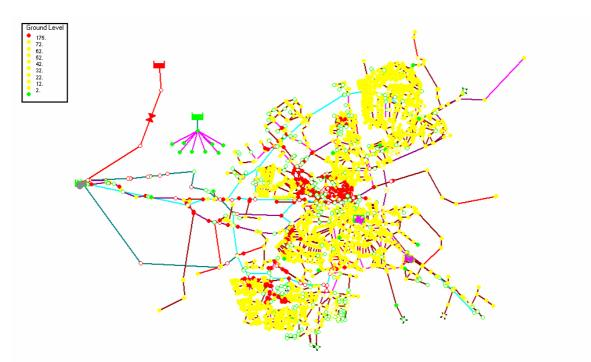
**Figure 2.3:** Calculated maximum concentrations when introducing a contaminant at the pumping station, reporting interval 30 minutes. The legend heading ground level should be replaced by concentration.
