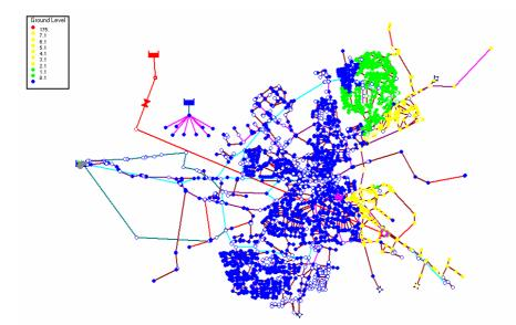
**Figure 2.10:** Calculated maximum concentrations when introducing a contaminant in the lower reservoir, reporting interval 30 minutes. The legend heading ground level should be replaced by concentration.
