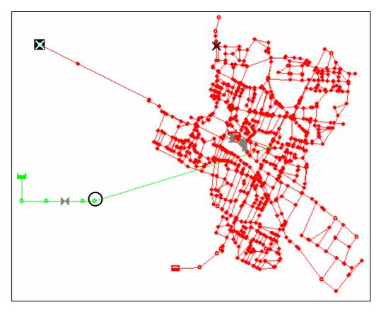
**Figure 2.12.** Overview of town B's water mains system and modelling of the injection of a toxic substance (see green node. The contamination is injected in the encircled node).
