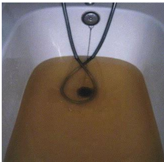
Figure 61 Discolouration in potable water distribution systems (Vreeburg and Boxall 2007).
