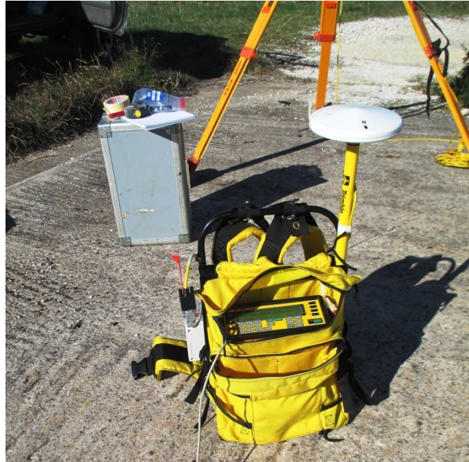
Figure 28. Rover Station, used to provide accurate coordinates to the GPR system
