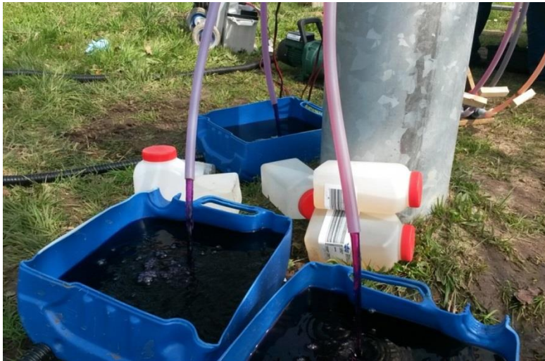
Figure 2-7 Purple water (due to the presence of MnO 4 ) pumped from the 3 screens of the monitoring well 5 m away from well 10.
