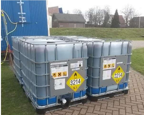
Figure 2-6 Four IBC's of sodium permanganate, dosed to the injected 2000m 3 during the second experimental cycle of well 10.
