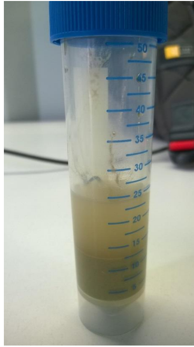
Figure 76: Abstracted water during clean pumping after 24 ha stand-still with Na-hypochlorite
