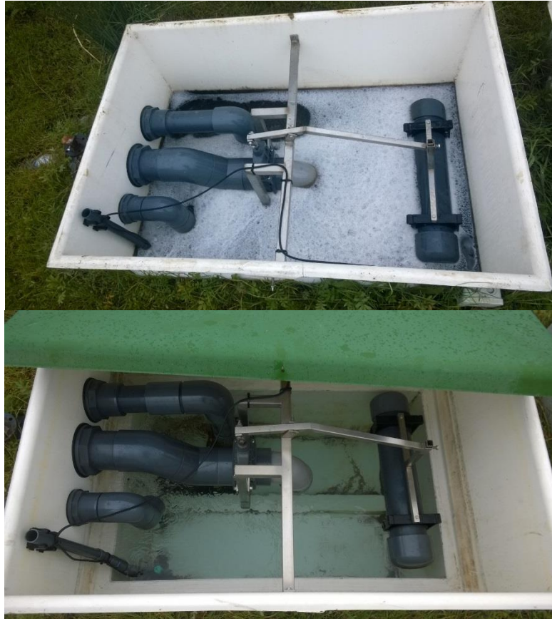
Figure 75: Floater box during and after the treatment with Na-hypochlorite.
