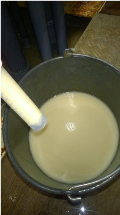
Figure 76: Abstracted water during clean pumping after 24 ha stand-still with Na-hypochlorite
