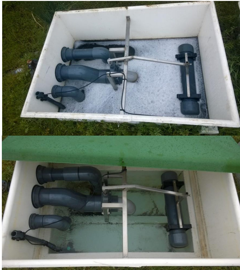
Figure 17.3: Floater box during and after the treatment with Na-hypochlorite.
