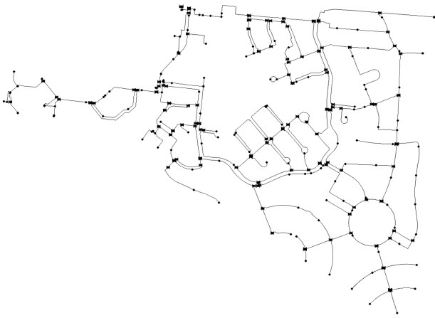
Figure 1. EPANET model of the drinking water distribution network of Sittard (Netherlands), consisting of 583 junctions, 491 pipes, 140 valves and 1 reservoir.
