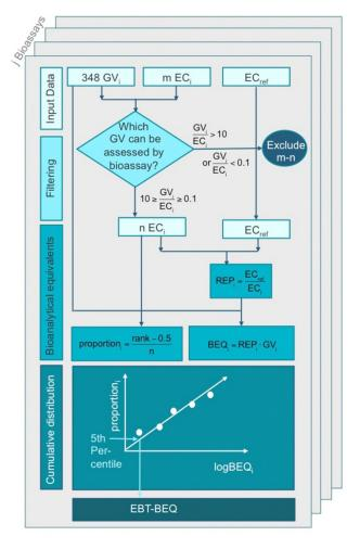
FIGURE 4.3. APPROACH TO DERIVE EBT-BEQS FOR CELL-BASED BIOASSAYS (GV = GUIDELINE VALUE, EC = EFFECT CONCENTRATION, BEQ = BIOANALYTICAL EQUIVALENT CONCENTRATION, REP = RELATIVE EFFECT POTENCY, N = NUMBER OF CHEMICALS I, M = NUMBER OF AVAILABLE EC VALUES PER BIOASSAY J, REF = REFERENCE COMPOUND) (ESCHER ET AL., 2015).
