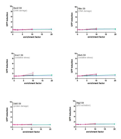
FIGURE S4.2. RESPONSES (MEAN±STDEV) INDUCED BY A SELECTION OF WATER SAMPLE CONCENTRATES (AT DIFFERENT FINAL ENRICHMENTS IN THE ASSAY) ON TOXTRACKER BIOMARKER GFP IN THE PRESENCE OF METABOLIC MIXTURE S9. BLUE: DRINKING WATER; GREEN: SURFACE WATER; PINK: WASTE WATER TREATMENT PLANT EFFLUENT.
