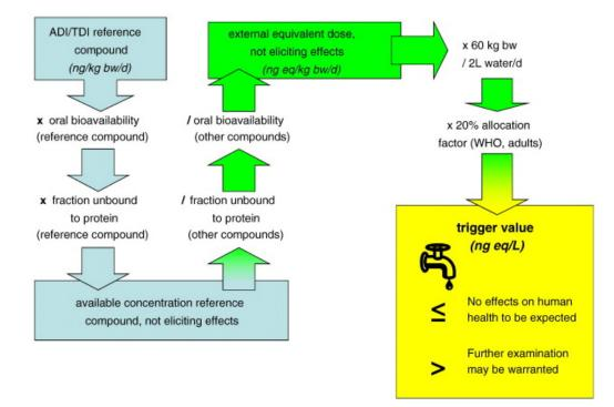
FIGURE 4.2. FLOW DIAGRAM OF DERIVING TRIGGER VALUES FOR ADDITIONAL INVESTIGATION FOR HORMONAL ACTIVITIES IN WATER FROM ACCEPTABLE OR TOLERABLE DAILY INTAKE (ADI OR TDI) VALUES OF REFERENCE COMPOUNDS (BRAND ET AL., 2013).
