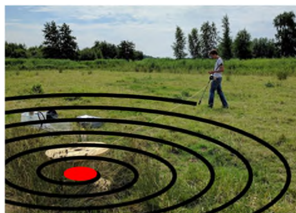
Fig. 2. Photo of the surficial scanning in action. Operator is attached to a wooden cylinder placed on the estimated location of the buried well, as marked with a red dot. The black line schematically shows the remaining path to be walked. (For interpretation of the references to color in this figure legend, the reader is referred to the web version of this article.)
