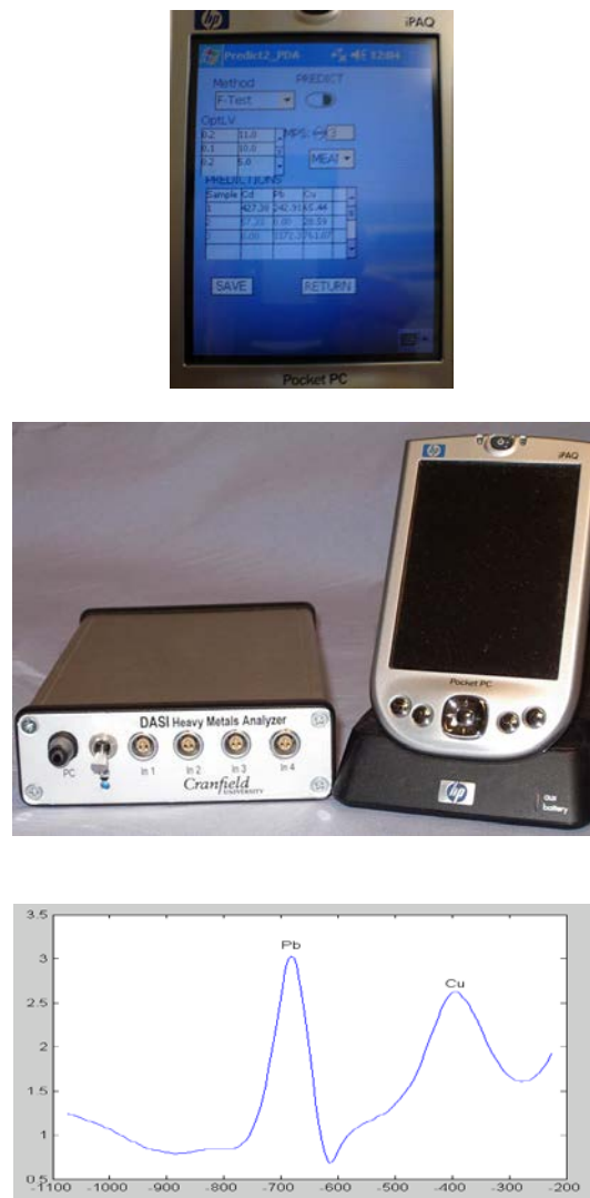
Figure 9: (upper) Metals analysis software loaded onto PDA; (middle) multiplex potentiostat; (below) typical voltammetric response for lead and copper using multiplex potentiostat.
