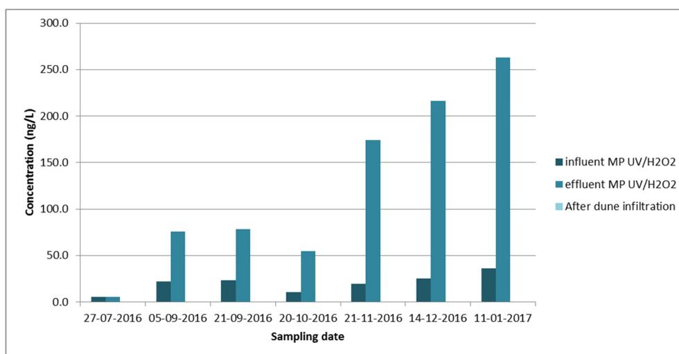
Figure 14: Summed concentrations of the detected by-products in the Heemskerk full-scale water treatment facility in influent MP UV/H<sub>2</sub>O<sub>2</sub>, effluent MP UV/H<sub>2</sub>O<sub>2</sub> and after dune infiltration water, analysed using the QToF N-DBP target method.
