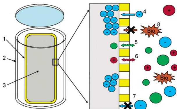
Figure 2-1: Schematic showing of the components of the passive sampler. (1) The 1000 kDa polyvinylidene fluoride membrane. (2) Porous HDPE casing. (3) DEAE-cellulose resin. (4) Negatively charged DOM enters the membrane and is retained and concentrated. (5+6) Dissolved neutral or positively charge analytes can enter the membrane but are not retained. (7+8) Large species cannot enter the membrane. Adapted from Lam and Simpson [44].
