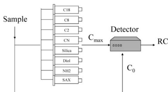
Figure 2-4: Experimental setup for PRAM (source: Rosario-Ortiz et al. [48]) The retention coefficient (RC) is calculated by means of the maximum breakthrough concentration and initial concentration. Other combinations of SPE cartridges can also be used in parallel.
