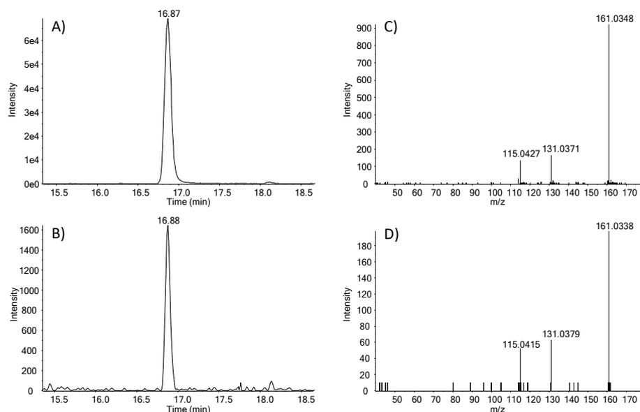
Figure 5: confirmation of N-DBP m/z 161.0360 in artificial water. A) EIC of m/z 161.0360 in Trp +  $^{14}\text{NO}_3^-$  after MP UV sample. B) EIC of m/z 161.0360 in artificial water after MP UV. C) MS2 spectrum of m/z 161.0360 in Trp +  $^{14}\text{NO}_3^-$  after MP UV sample. D) MS2 spectrum of m/z 161.0360 in artificial water after MP UV.
