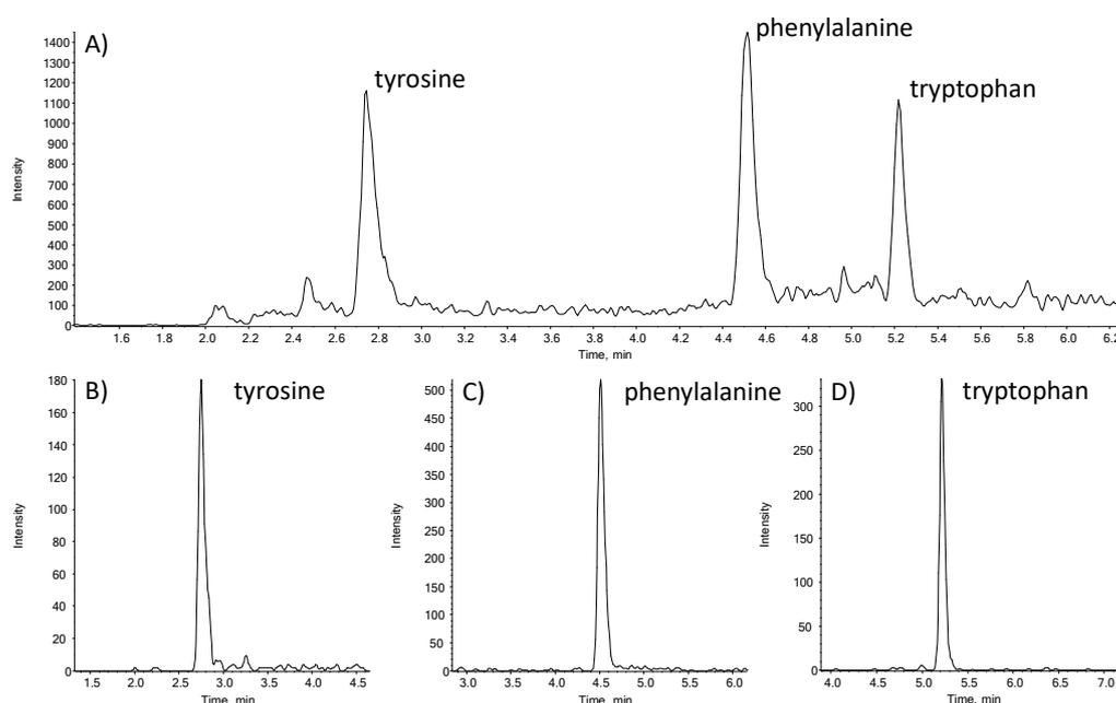
Figure 2: Chromatograms of drinking water spiked with 0.25 µg/L aromatic amino acids. A) Summed EIC  $[M+H]^+$  trace (10 ppm) of aromatic amino acids. B) Tyrosine MS2 EIC of  $m/z$  91.0542. C) Phenylalanine MS2 EIC 120.0808. D) Tryptophan MS2 EIC of  $m/z$  118.0651.
