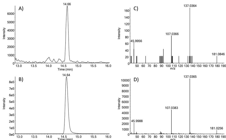
A) EIC of  $m/z$  181.0255 in artificial water after MP UV. B) EIC of 2-Amino-3-nitrobenzoic acid reference standard ( $m/z$  181.0255). C) MS2 spectrum of  $m/z$  181.0255 in artificial water after MP UV. D) MS2 spectrum of 2-Amino-3-nitrobenzoic acid reference standard.
