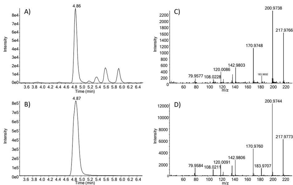
A) EIC of  $m/z$  217.9765 in artificial water after MP UV. B) EIC of 4-hydroxy-3-nitrobenzenesulfonic acid reference standard ( $m/z$  217.9765). C) MS2 spectrum of  $m/z$  217.9765 in artificial water after MP UV. D) MS2 spectrum of 4-hydroxy-3-nitrobenzenesulfonic acid reference standard.
