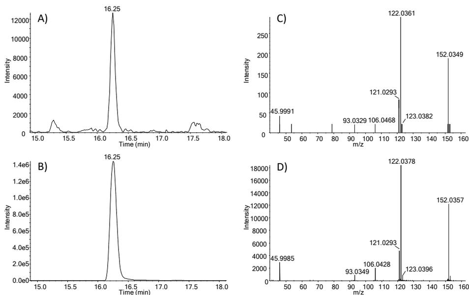
A) EIC of  $m/z$  152.0353 in artificial water after MP UV. B) EIC of 2-methyl-4-nitrophenol reference standard ( $m/z$  152.0353). C) MS2 spectrum of  $m/z$  152.0353 in artificial water after MP UV. D) MS2 spectrum of 2-methyl-4-nitrophenol reference standard.
