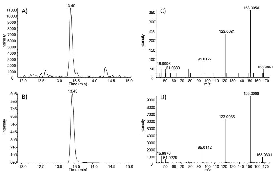
A) EIC of  $m/z$  168.0302 in artificial water after MP UV. B) EIC of 2-methoxy-4-nitrophenol reference standard ( $m/z$  168.0302). C) MS2 spectrum of  $m/z$  168.0302 in artificial water after MP UV. D) MS2 spectrum of 2-methoxy-4-nitrophenol reference standard.
