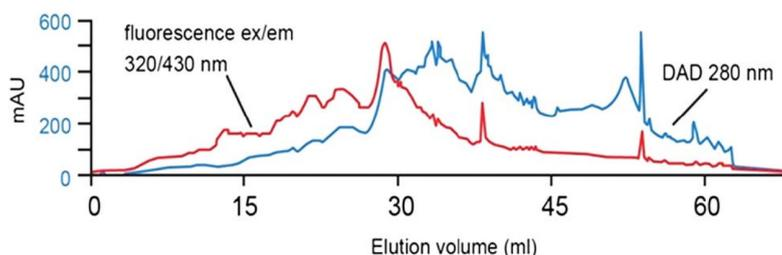
Figure 4-3: HILIC chromatogram of Suwannee river DOM recorded using DAD (blue) and fluorescence (red) detection. Source Sandron et al. [43] and Woods et al. [88].
