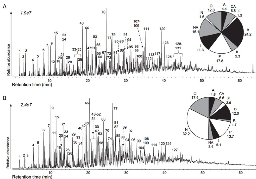
Figure 4-4: MSSVpy TIC GC-MS data of the HPO fraction (A) and HPI fraction (B). The pie chart reflects relative proportions of ten major groups. A = aliphatic, CA = cycloaliphatic, F = Furans, B = benzenes, K = ketones, P = phenols, I = indenes, NA = naphthalenes, N = nitrogen products and O = other. Adjusted from Berwick et al. [173].
