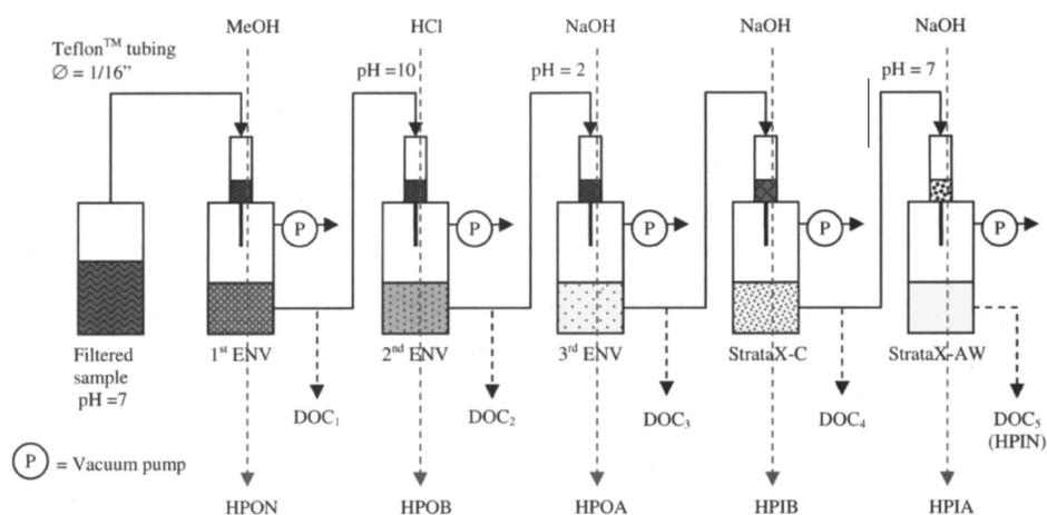
Figure 2-3: SPE fractionation setup and procedure for obtaining six fractions. Source Ratpukdi et al. [70].
