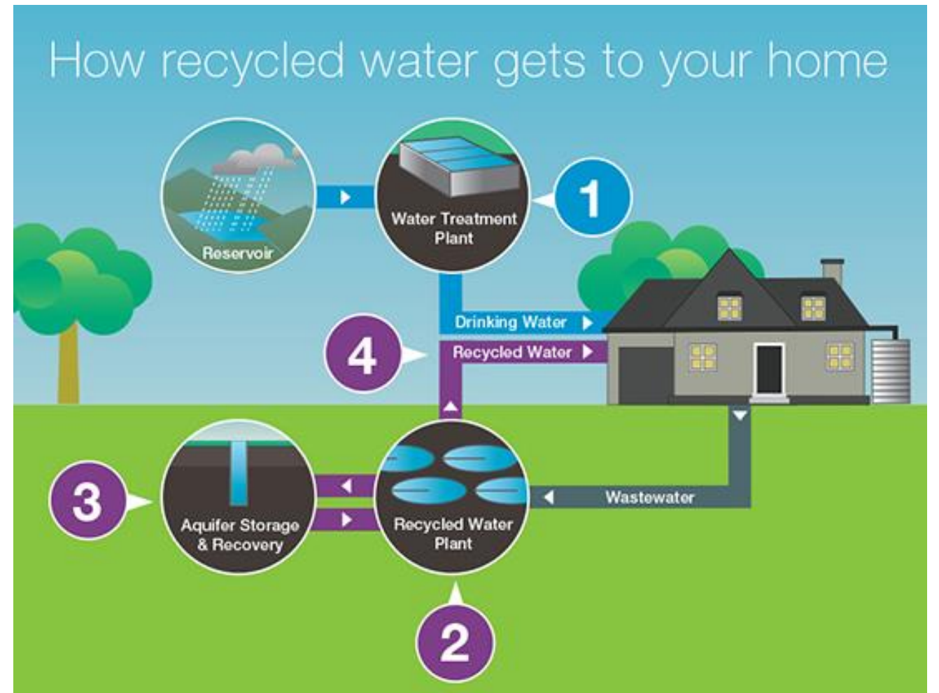
City West Water, Melbourne: waste water reuse upon aquifer storage for non-potable water
