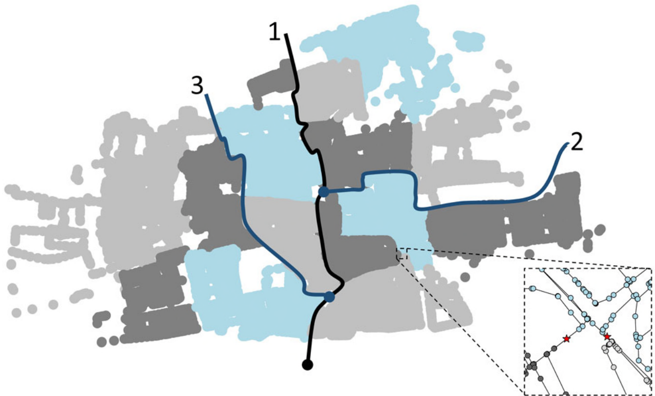
Figure 2. The selected DMA configuration for The Hague. The different coloured boxes represent different DMAs. The three numbered lines represent the first three of eight steps that comprise the optimal transition to this configuration. The magnified part of the water supply grid shows several boundaries between DMAs, marked with a star.
