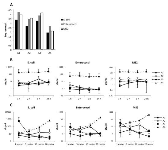
**Figure 4.** (**A**). Flushing efficacy (A1–A3: 1.27 m/s; 2.5 volumes; A4: 0.45 m/s, 0.9 volumes) of the individual experiments. (**B**) Role of waiting time after flushing (**C**) and distance from the contamination point on the number of microorganisms in the water. Shown is the average, with SD, of the results of four distances per time point (**B**) or the average of the results of four time points per distance point (**C**).
