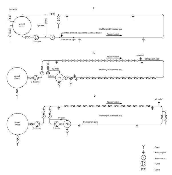
**Figure 1.** Schematic overview of the pipe-loop distribution systems that were used for experiments A1–A4 (a), B1–B3 (b) and B4, B5, C1–C3 (c). In systems B and C pipe segments were placed between valves that were replaced with new segments to sample the biofilm.
