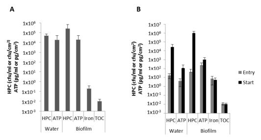
**Figure 3.** Average (with standard deviation (SD)) of heterotrophic plate count (HPC) number, adenosine triphosphate (ATP) and iron concentration of the cultured biofilm after 14 days (( $\mathbf{A}$ ), n = 2-5) and, including TOC levels, of natural biofilms upon arrival at the laboratory (entry) and immediately before start of the experiment (( $\mathbf{B}$ ), n = 3).
