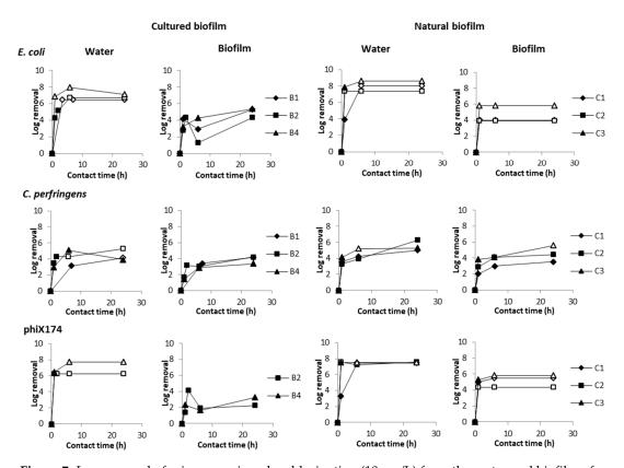
**Figure 7.** Log removal of microorganisms by chlorination (10 mg/L) from the water and biofilm of a cultured and natural biofilm in log removal. Markings in white indicate a result below the detection limit and is thus a '>value' in log removal.
