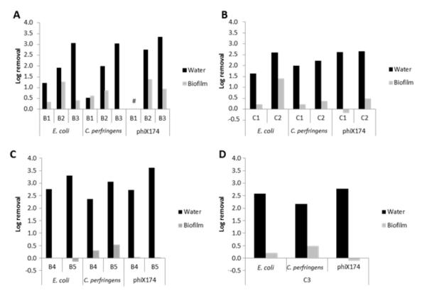
**Figure 5.** Flushing efficacy in log removal of microorganisms from the water and biofilm of a pipe with a cultured biofilm (**A**,**C**) or a natural biofilm (**B**,**D**). In (**A**) (experiments B1–B3) and (**B**) (experiments C1–C2) the pipe-loop system was flushed with 3 volumes at 1.5 m/s. In (**C**) (experiment B4–B5) and (**D**) (experiment C3) the pipe-loop system was flushed with 3 (water) or 15 volumes (biofilm) at 0.3 m/s. # phiX174 not added to pipe-loop system and not determined.
