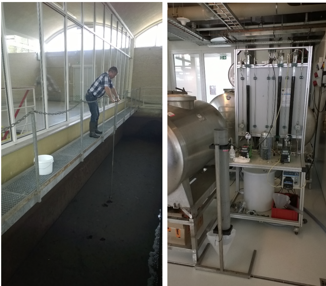
FIGURE 4A. SAMPLING OF RSF FILTERS AT WRK NIEUWEGEIN (WATERNET). B. COLUMN SETUP USED IN RSF LAB-SCALE EXPERIMENTS.
