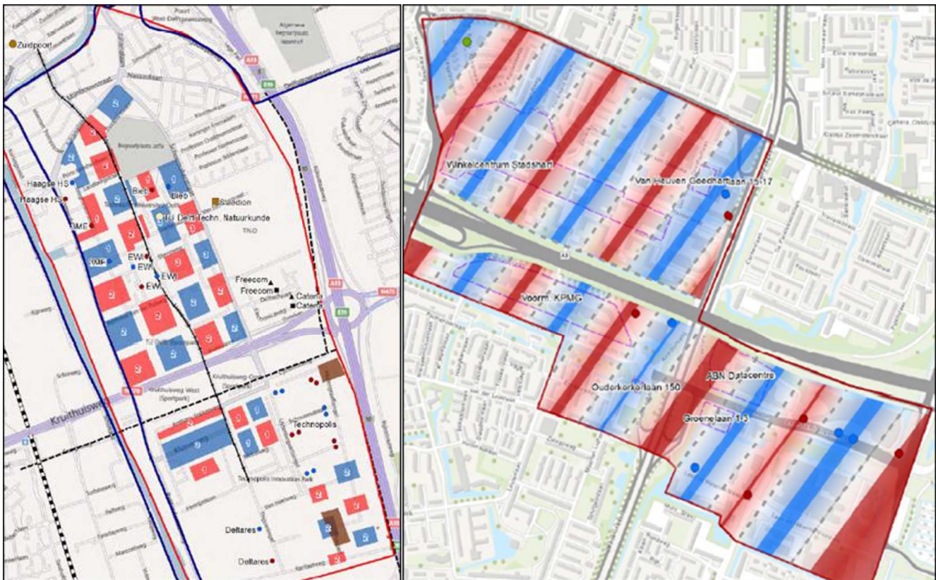
Fig. 1. A cut out of the ATEs plan maps in Delft (left) and Amstelveen (right), indicating search areas for warm and cold well (the red and blue areas) and existing well locations (green, red and blue markers). (For interpretation of the references to color in this figure legend, the reader is referred to the web version of this article.)
