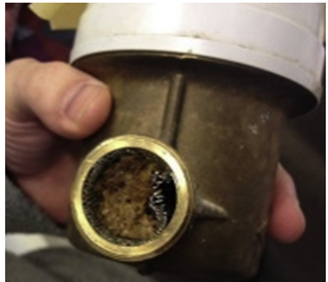
Fig. 4. Picture of particulate matter that clogged the water meter in Oasen's Hendrik Ido Ambacht supply area.
