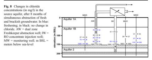
SEAWAT modelling suggested that the brackish water abstraction rate can be lowered to  $16 \text{ m}^3$ /h to keep chloride concentrations in the abstracted freshwater well constant at 45 mg/L.
