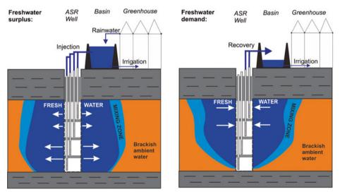
Fig. 3 Use of multiple partially penetrating wells (MPPW) for improvement of freshwater recovery of coastal ASR systems storing rainwater harvested from greenhouse roofs
