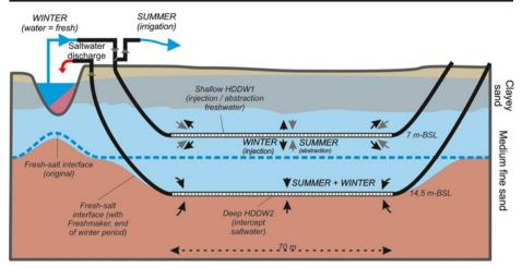
Fig. 6 Use of the Freshmaker principle to enlarge freshwater lenses. Side-view at the HDDWs. Set-up as installed at the Ovezande field-trial. m-BSL = meters below sea-level
