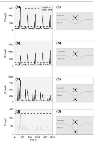
risk for the salinity of the abstracted water. The simulation results show the upper part of the aquifer will gradually freshen, which will result in a decrease in saline seepage towards a local water course and eventually even local infiltration via the water course during freshwater recovery.
