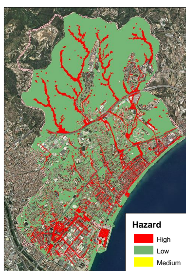
Figure 176. Pedestrian hazard map of Badalona obtained from simulation of an extreme rainfall event registered 15 km away from Badalona.
