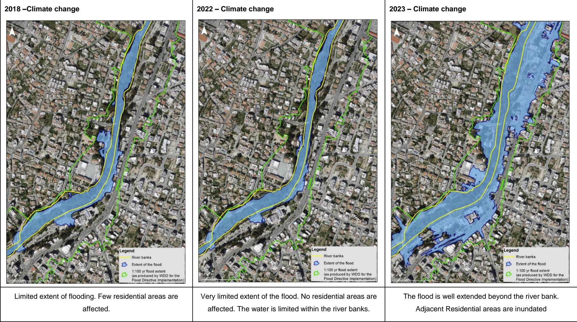
Figure 20: Flood Map at a selected indicative residential area of the examined flood events (most extreme ensemble member) under climate change scenarios
