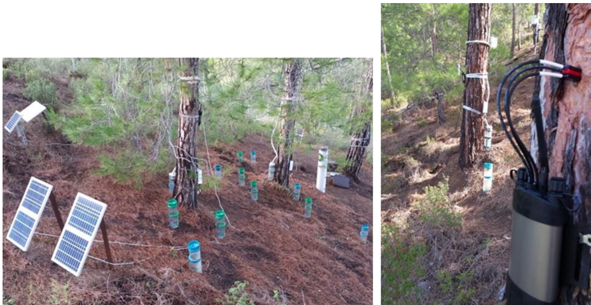
Figure 3.2 Pinus brutia trees, sap flow sensors, soil moisture sensors, throughfall gauges at the Agia Marina_Xyliatou forestry research site.
