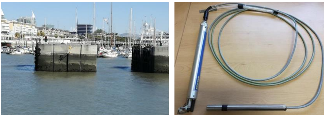
Figure 7.2 General overview of the Parque das Nações station and SEBA MPS D3 multiparameter probe with SEBA Slimcom2 data logger.
