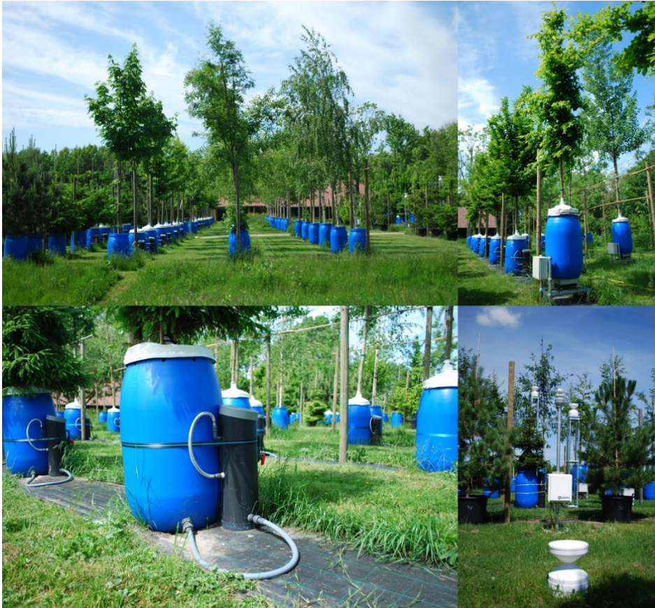
Figure 5.3 Overview of the experiment at KWR with the individual trees in pots, the high resolution weighing balances, the water supply device and the meteorological station.
