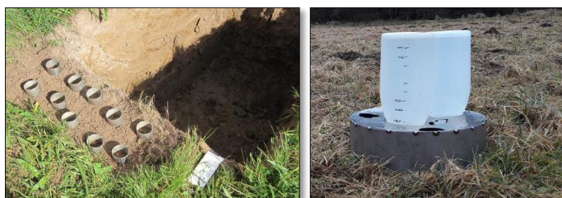
Figure 4.5. Samples and double-ring infiltrometer test
