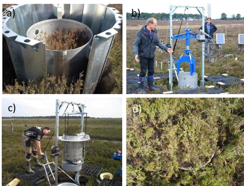
Figure 5.1 Installation of one of the lysimeters at the Hoge Veluwe.
