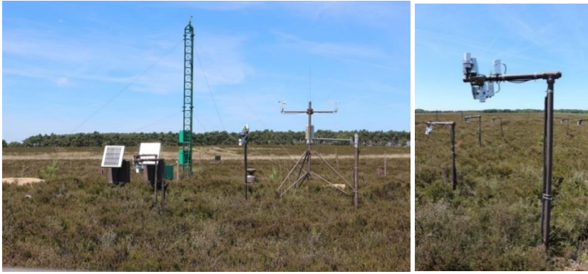
Figure 5.2 Overview of the field station (left) and infra-red sensors for surface temperature.
