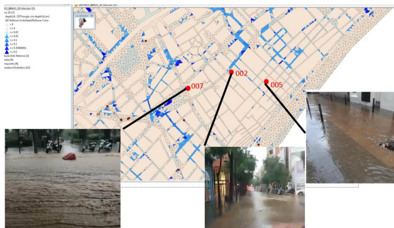
Figure 8.3. Visual surface flood calibration process using photos and videos. Event of July 2018
