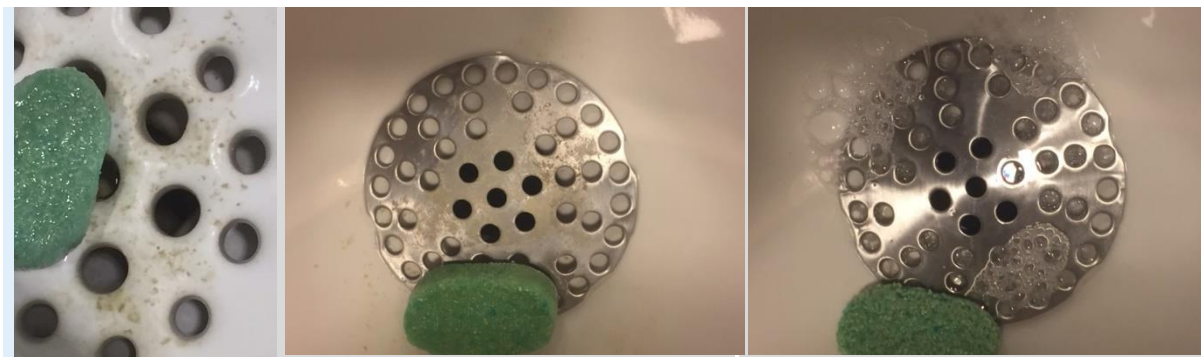
Figure 26: Adsorbent attached to ceramics and metal. Left and middle picture before cleaning, right picture after cleaning.
