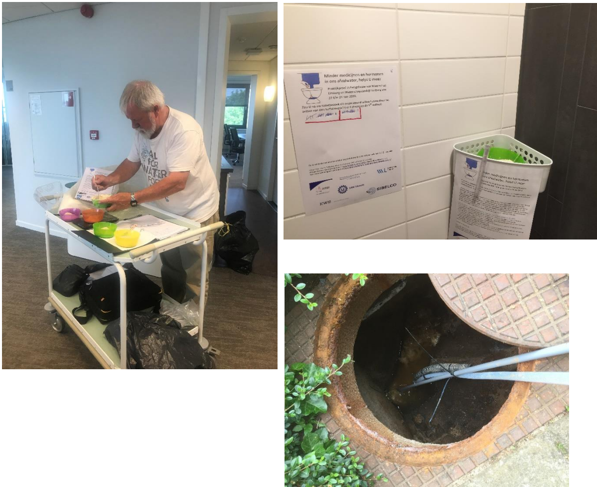
Figure 24: Pilot investigation at WL/WBL in Roermond. Left: weighing the powder for each toilet/container. Upper right: a tally sheet and the container with the powder and the small spoon. Lower right: sampling in the sump in the Kapelaan Sarsstraat (old building)
