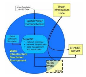
Figure 15: WISE Analytic Framework graphical representation (McPherson and Burian, 2005)
