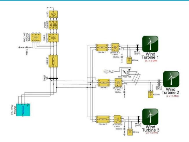
Figure 19: SCADASIM interface with connected elements of the model (Queiroz et al., 2011)
