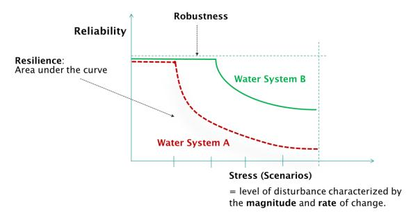
Figure 22: The concept of resilience profile graph (Makropoulos et al, 2018)
