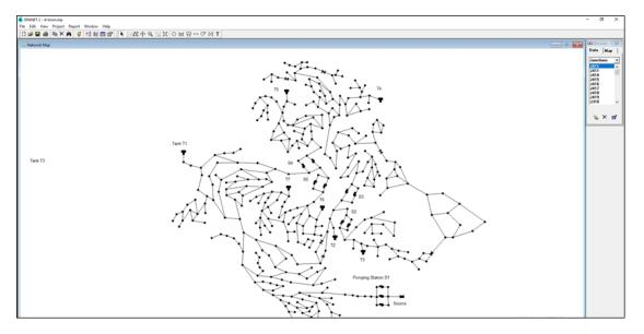
Figure 20: EPANET interface with C-Town network example
