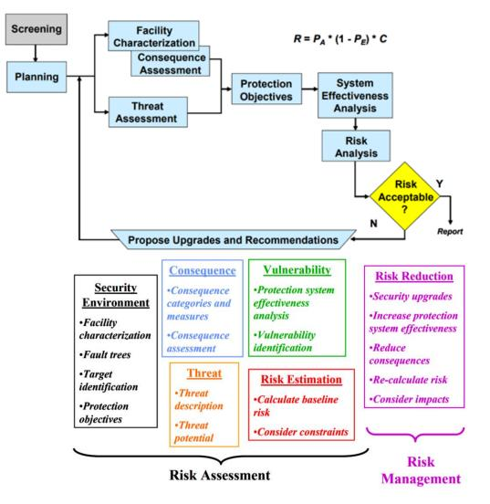
Figure 11: (a) Risk Assessment Methodology Process Flow Diagram (b) Major Modules in Risk Assessment & Treatment (Jaeger et al., 2008)
