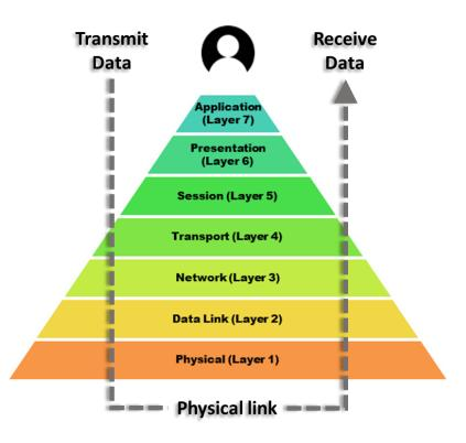
Figure 5: OSI architecture of 7 layers visualization
