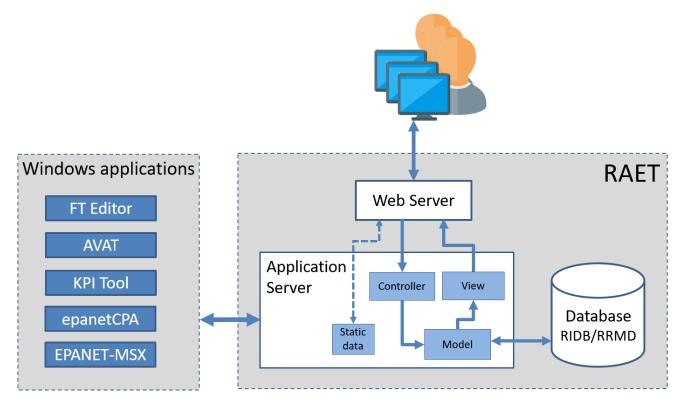
Figure 50: System architecture of RAET
