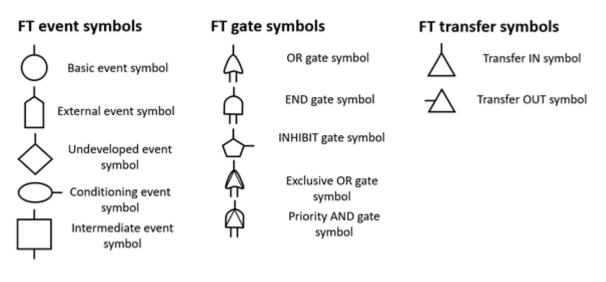
Figure 12: Commonly used symbols in the visualization of Fault Trees
