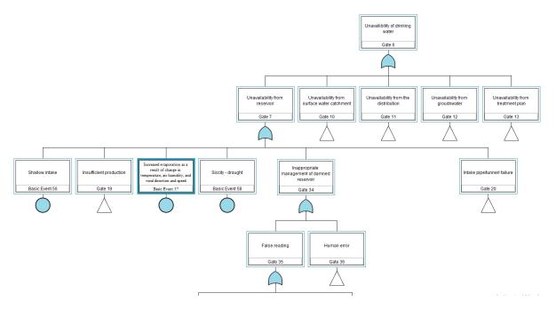
Figure 13: Part of the "unavailability of drinking water" FT created in PREPARED project, with a basic event highlighted
