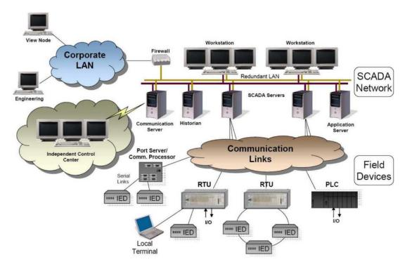
Figure 1: SCADA architecture (Queiroz et al., 2011)
