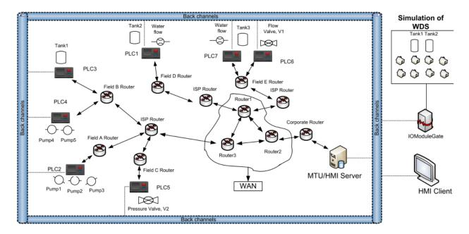
Figure 18: SCADAVT schematic of cyber layer assets and WDN connection (Almalawi et al., 2013)
