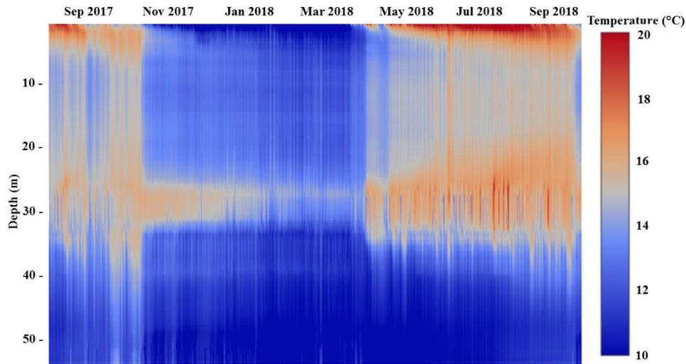
Figure 8. Temperature distribution in monowell (ATES-3) from September 2017 to October 2018. Scale bar (right) shows temperature range in °C. The positions of the warm (26 – 31 m bsl) well and cold well (49 – 56 m bsl) can be seen.
