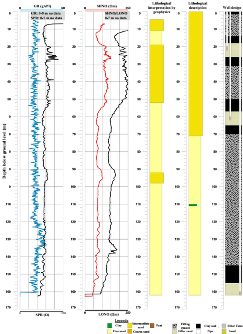
Figure 5. Illustration of combined geophysical measurements resulting in a soil profile and a well design. GR=Gamma Radiation; SPR=Single Point Resistance; SHNO=Short Normal; LONO=Long normal.
