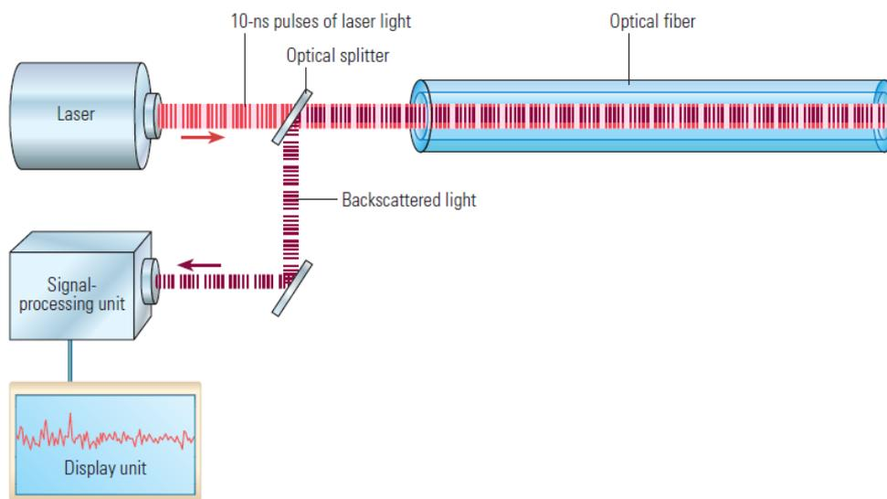
Figure 3. Temperature monitoring with fibre optics using raman backscatter DTS sensing.
