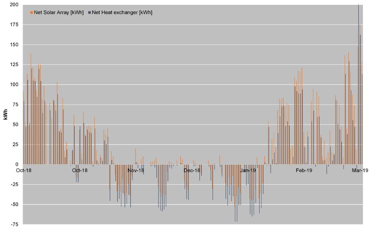
Figure 13. The measured “net energy” in Delft (like in Figure 12, measured at the thermal array and at the heat exchanger) which integrates the power over 24 hours and includes the frost-prevention approach of circulating water at night, so the figure shows the true total energy delivered by the PVT-system to the ATES / climate control system.
