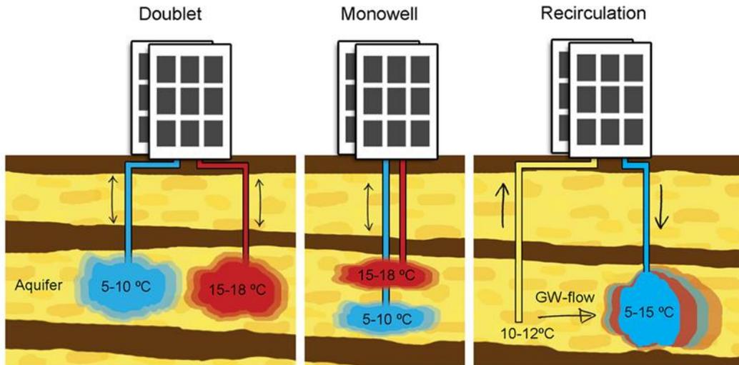
Figure 1. Schematic representation of ATES doublet, monowell and recirculation systems. The doublet system at the left is the most common. The monowell system in the middle, with the hot well on top of the cold well needs less space and has lower installation costs, since one borehole suffices. The recirculation system is preferable at high groundwater flows but is less effective, since infiltrated cold and heat are not reused.
