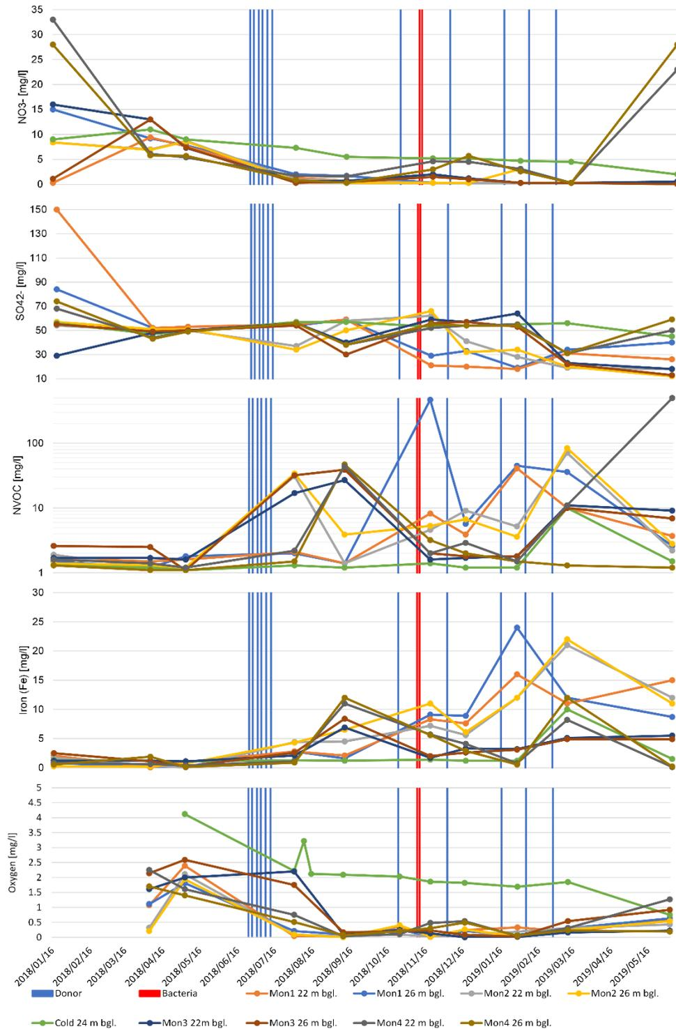
Figure 14. Following electron donor additions into the hot well at the Danish site, organic matter (NVOC) and dissolved iron concentrations increase in all monitoring wells, while electron acceptors oxygen, nitrate and sulphate concentrations decrease. Monitoring wells 1,2, 3 and 4 are situated on a straight line between the hot and the cold well.
