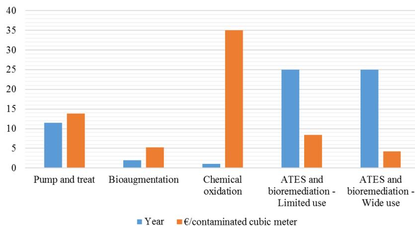
Figure 17. Results of the economic comparison of different groundwater remediation technologies: treatment duration and discounted cost per cubic meter of contaminated groundwater for pump and treat, bioaugmentation, chemical oxidation and ATES+bioremediation.
