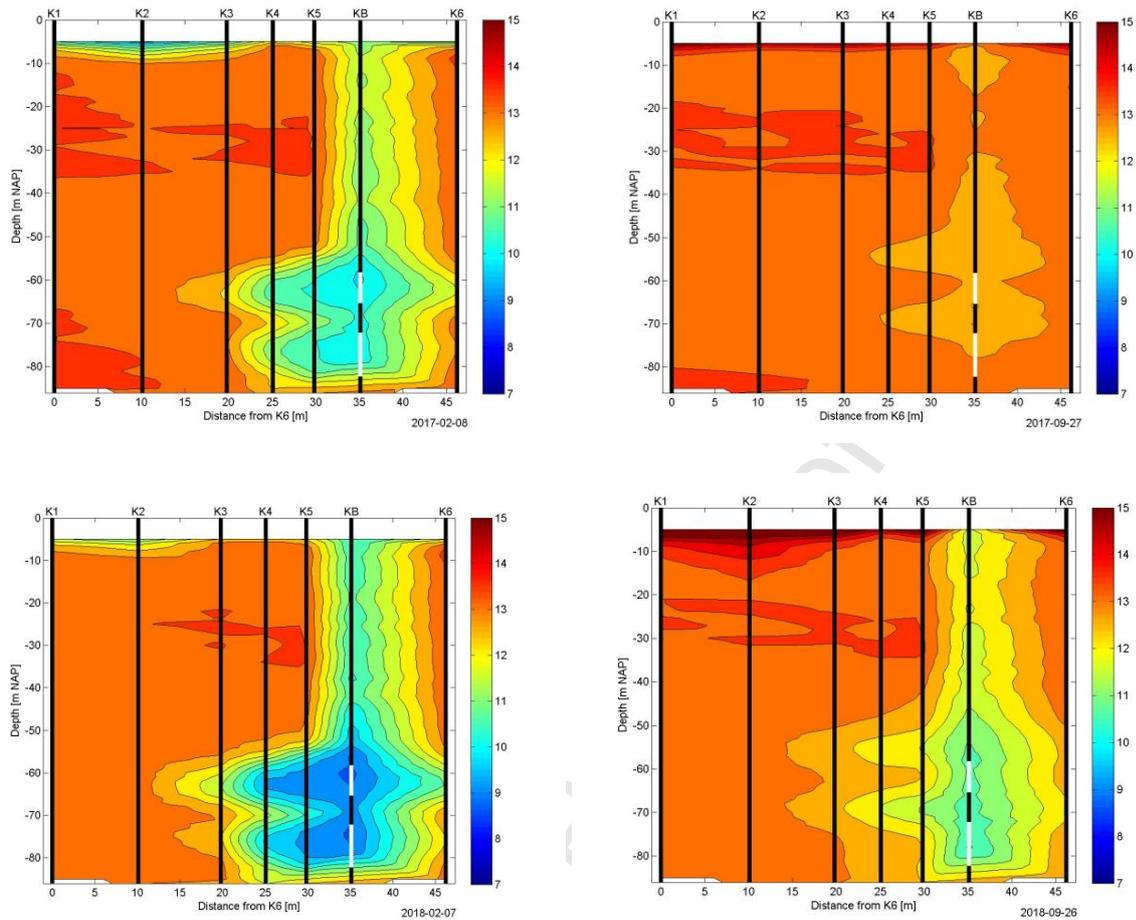
Figure 10. Spatial temperature measurements in Delft (Netherlands), derived from high resolution measurements in glass fiber cable at 6 distances around the cold well. See also motion pictures published on-line.
