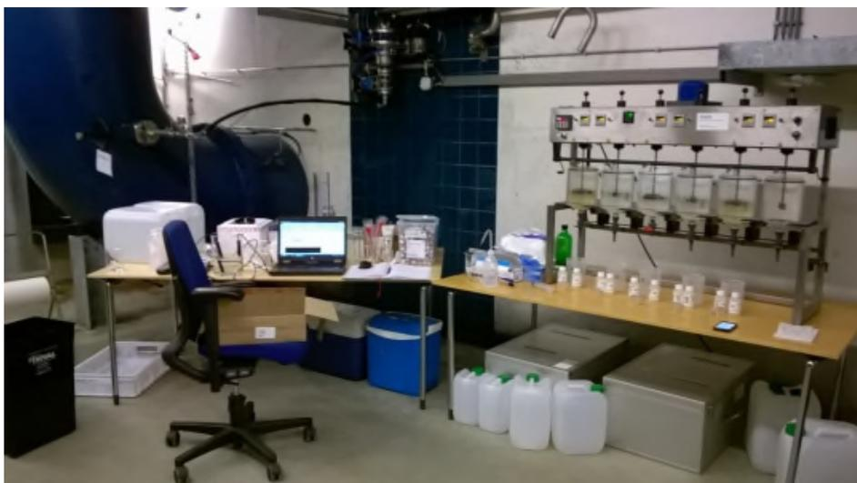
FIGURE 2-2 JAR TESTING SETUP AT DWTP KATWIJK.
