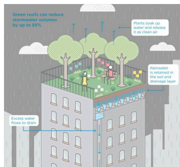
Figure 4 Example of how a green roof can reduce stormwater volumes by up to 85% (City of Melbourne, n.d.)
