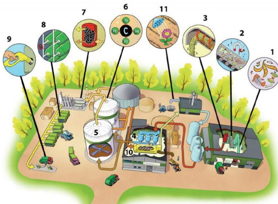
Figure 11 Illustration of how food waste is processed into biogas and biofertilisers in Stockholm (Scandinavian Biogas, n.d.)
