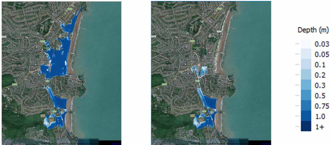
Figure 9 | Flood extents of a 1 in 200-year coastal overtopping event with 50 years climate change: (left) no sea wall, (right) sea wall option.
