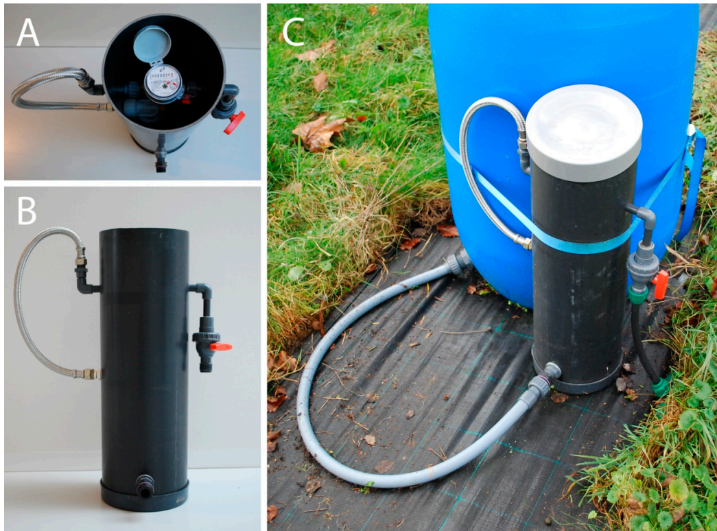
Figure 2. Water supply device. (A) View from above on the water meter (float valve positioned underneath). (B) View from the front. (C) Field installation.
