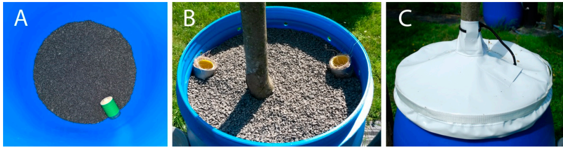
Figure 3. Plant container preparation. (A) Nozzle and gravel in the lower part of the container. After the picture was taken, more gravel was added until the nozzle was covered. (B) Gravel covering the soil surface. The ends of the drainage pipe as well as the ventilation holes near the rim of the container are visible. (C) Rain cape.
