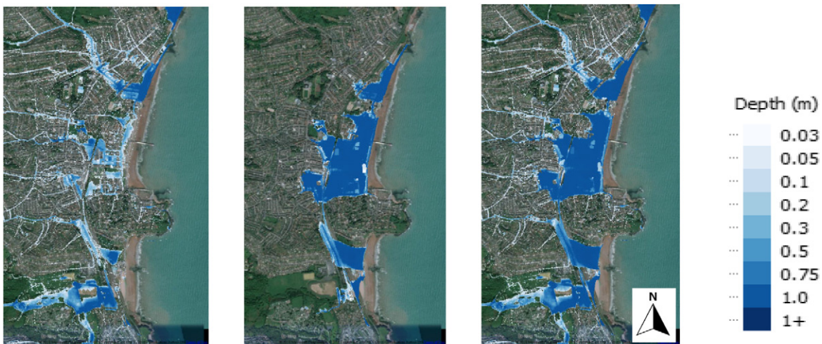
Fig. 8. Flood extents of 1 in 100 year return period pluvial event (left) and 1 in 200 year return period overtopping event (centre), and combined 1 in 50 year pluvial and coastal overtopping event (right), each for the 50 years of climate change scenario.
