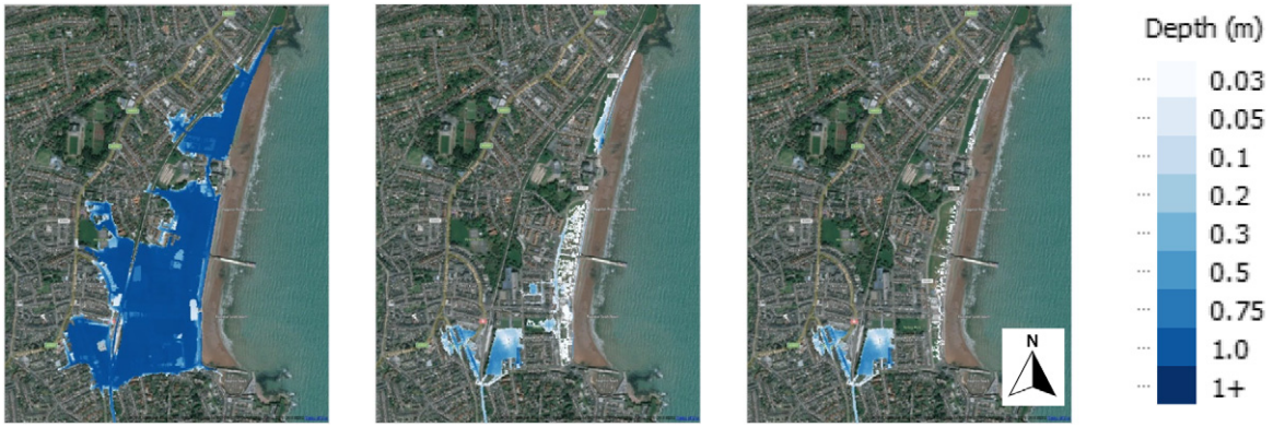
Fig. 9. Flood extents of 1 in 200 year coastal overtopping event with 50 years of climate change: (Left) no sea wall, (Centre) Smallest wall option, (Right) Largest wall option.
