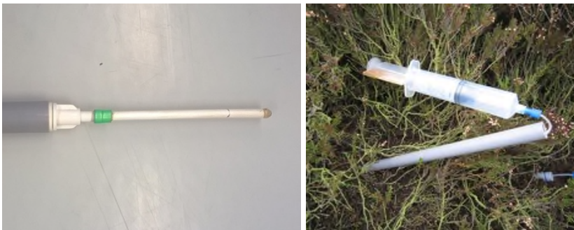
Figure 3. Soil water sampler 'macrorhizons' (left) and their installation in the field (right).
