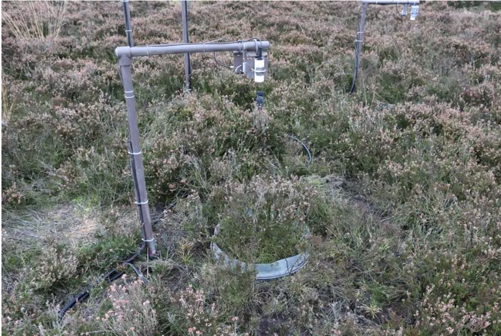
Figure 2. Precision lysimeters installed in the study site.
