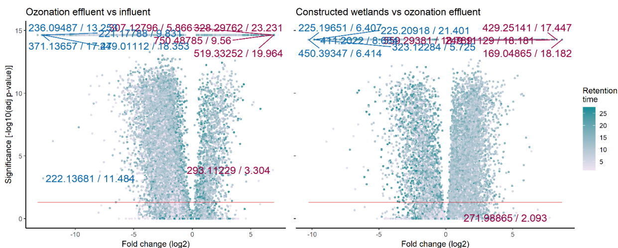
FIGURE 15 COMPARISON OF FEATURE INTENSITIES BETWEEN OZONATION EFFLUENT AND INFLUENT (LEFT PANEL) AND OZONATION EFFLUENT AND CONSTRUCTED WETLANDS (RIGHT) SAMPLES (APRIL SAMPLING ROUND). THE CHANGES BETWEEN FEATURE INTENSITIES (LOG2 FOLD CHANGE, X-AXIS) ARE PLOTTED AGAINST THE SIGNIFICANCE (P-VALUE) IN A VOLCANO PLOT. THE FIVE MOST INTENSE FEATURES OF THE RESPECTIVE BEFORE (BLUE) AND AFTER TREATMENT SAMPLES (RED) ARE LABELLED. THE FEATURES ARE COLOURED ACCORDING TO THEIR RETENTION TIME AS A MEASURE FOR POLARITY.
