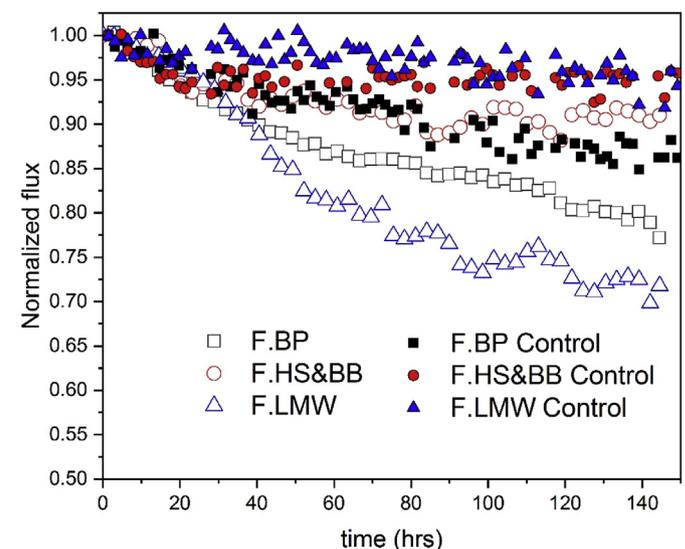
Fig. 6. Flux decline profile of RO biofouling by *Vibrio* sp. B2 (Kim and Chong, 2017) in different isolated dissolved organic fractions from seawater. The control experiments were tests without the presence of bacteria, taken from our previous work (Yin et al., 2019). Concentration of organic in each fraction = 0.5 mg-C/L. Initial flux = 30 L/m<sup>2</sup>h.
