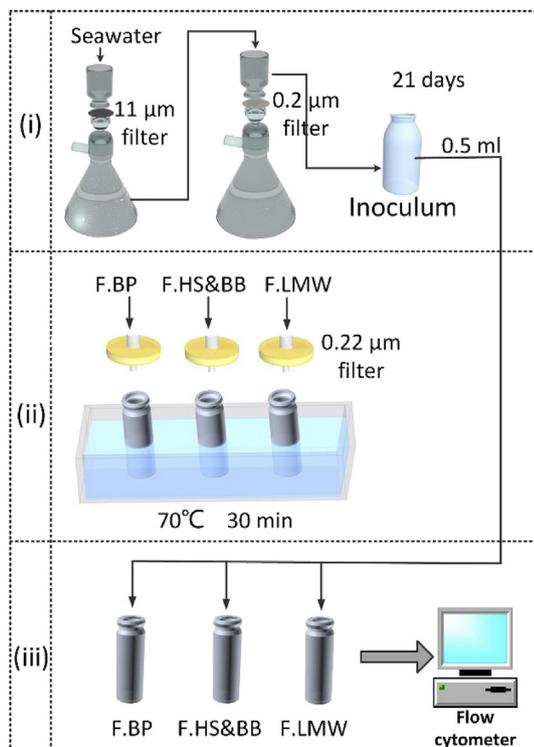
Fig. 1. The illustrations of (i) inoculum preparation, (ii) sample preparation and (iii) cell count measurement in AOC analysis.
