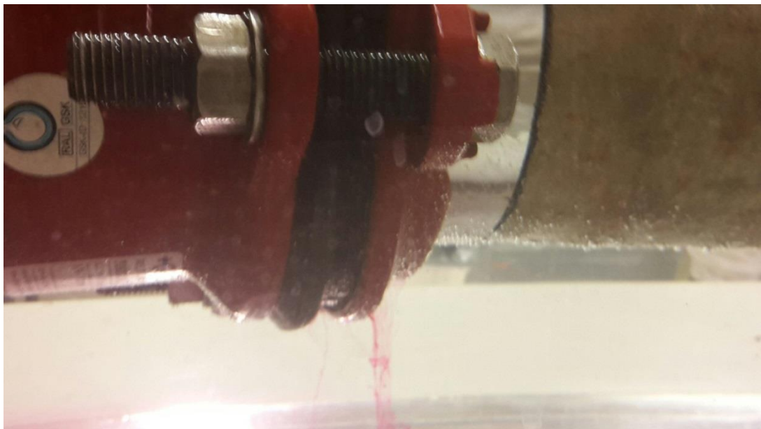
Figure 3.2.7.2: The leaching of the connected joint.
