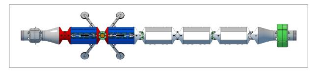
Figure 2: CAD model representing the selected design concept. From the left to the right, the following modules are present: propulsion + vision, centering (2x), battery/electronics (3x), propulsion + vision.
