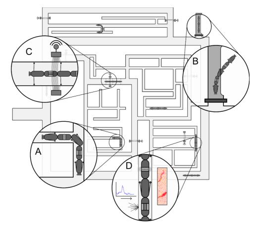
Figure 1: Vision of a system of autonomous robots that can freely move through the network (A), with access points for maintenance (B), facilities for energy and data transfer at several locations in the network (C), that is fitted with relevant sensors for pipe condition assessment, leak detection,
