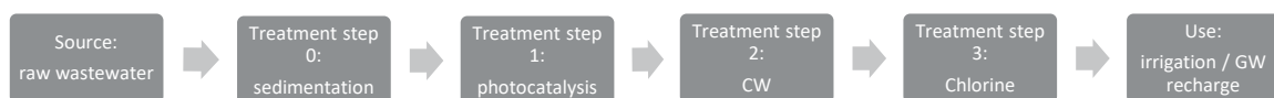
Figure 7 Simplified treatment scheme of site 10A - Water quality can be assessed after each step
