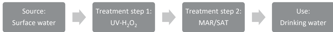
Figure 6 Simplified treatment scheme of site 6 - water quality can be assessed after each step
