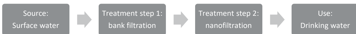
Figure 5 Simplified treatment scheme of site 1 - Water quality can be assessed after each step
