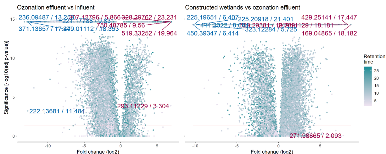
Figure 8 Comparison of feature intensities between ozonation effluent and influent (left panel) and ozonation effluent and constructed wetlands (right) samples (April sampling round)
